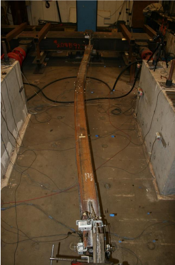
First peak compression, specimen buckling west east: cycle 21.5
