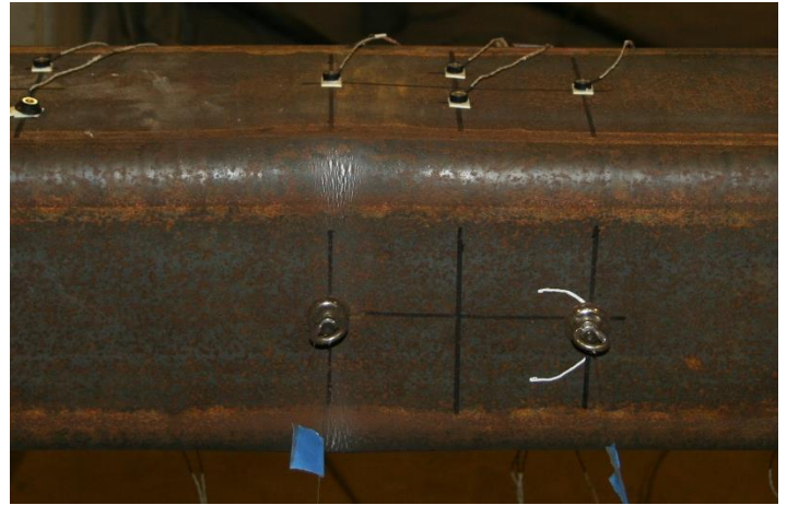
Striations forming on the corners of the east wall: cycle 17
