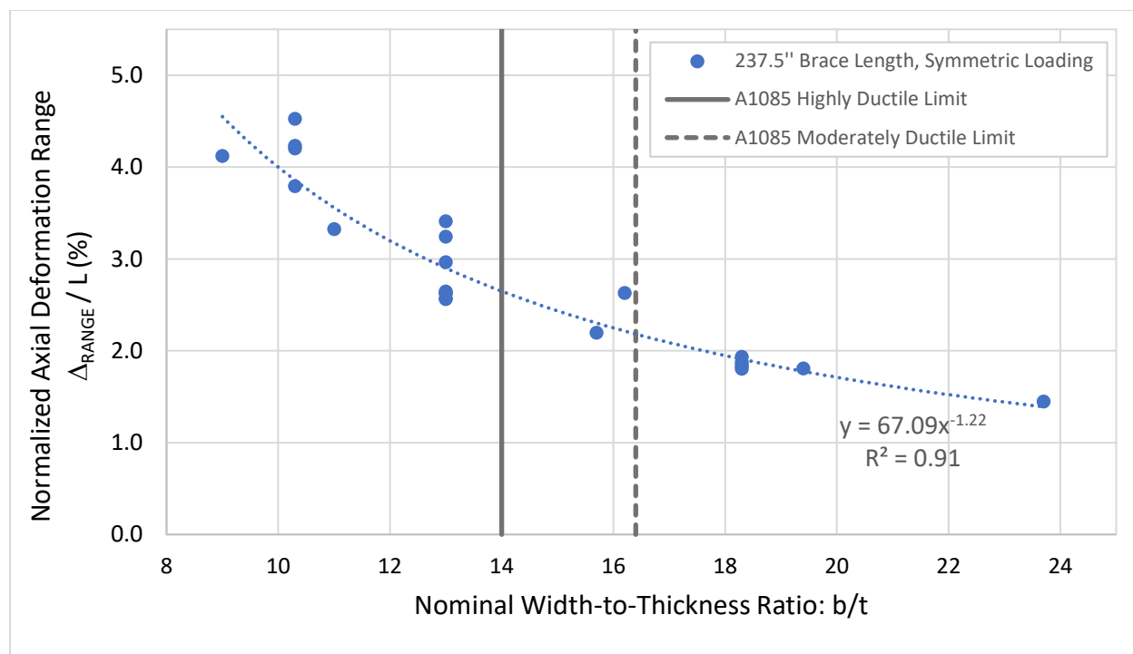
Figure 5.13 Axial Deformation Range vs. Local Compactness – Long Braces
