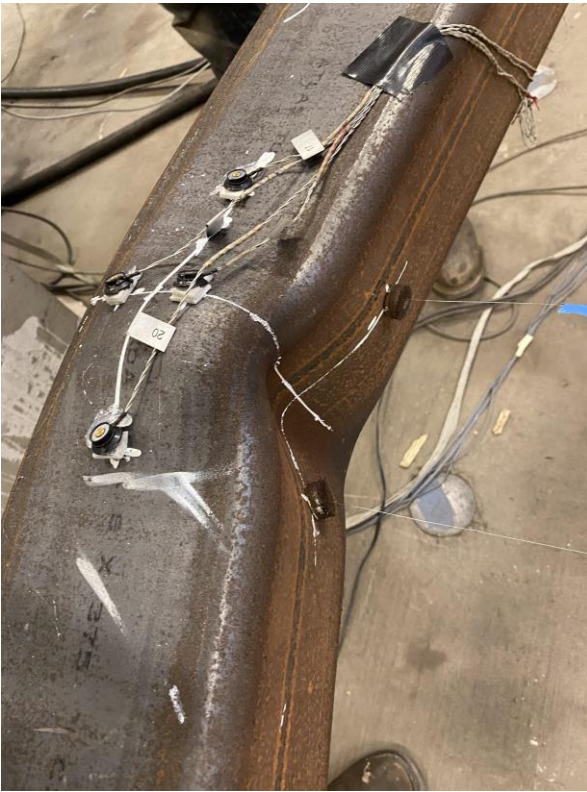
Cupping at Center of Specimen: 3.75" Cycle 1
