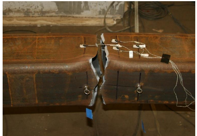
Specimen fractured at first 2.75" tension cycle
