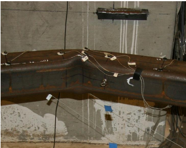
Cupping at peak out of plane displacement: Cycle 48
