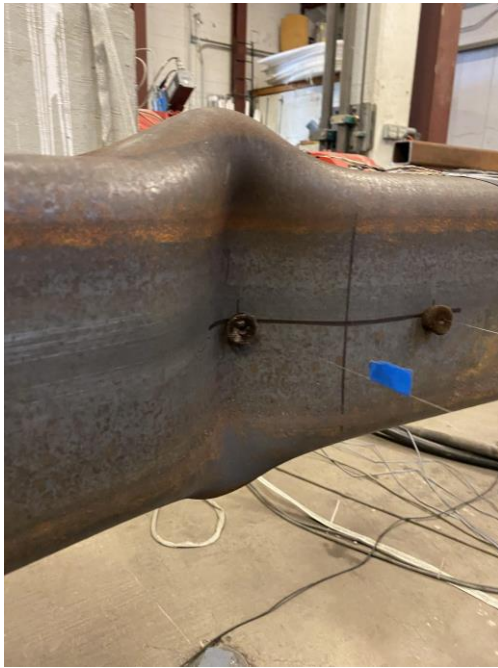
Cupping at Center of Specimen: 2.25" Cycle 1 C
