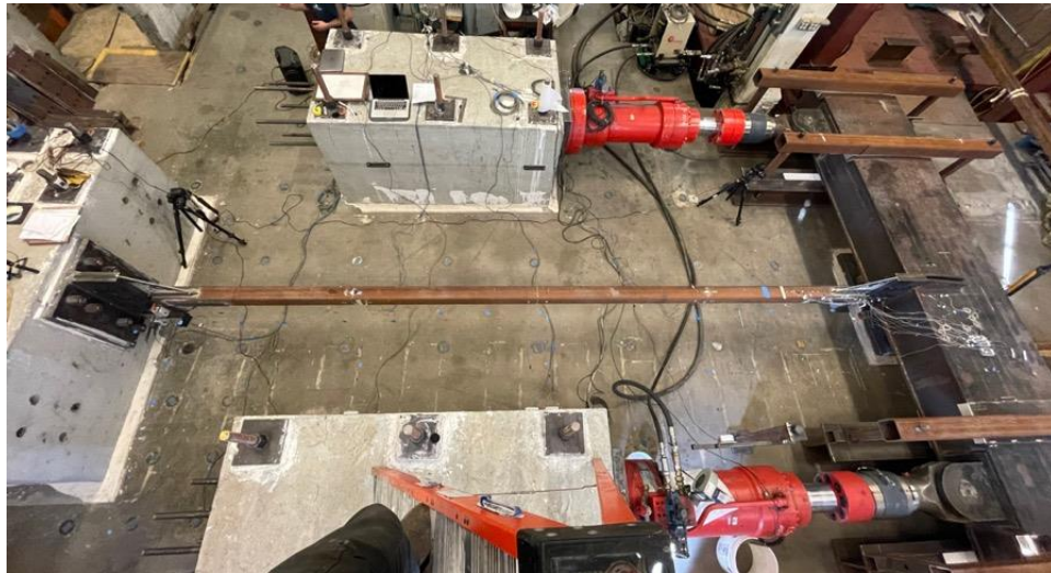
Figure 3.3. Configuration of Test Frame for 237.5" Brace Specimen
