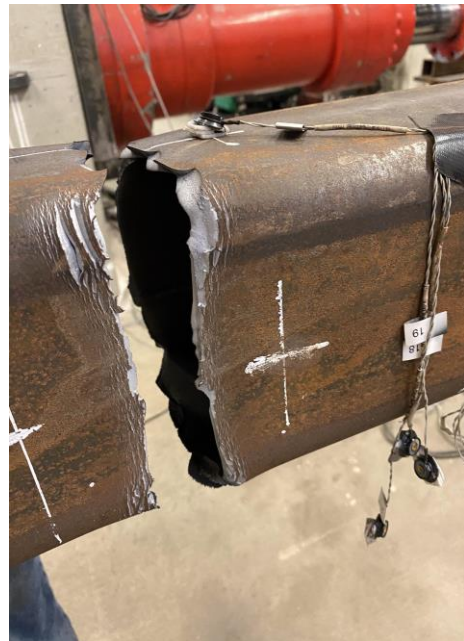
Fractured Specimen: First Cycle at 4.25"
