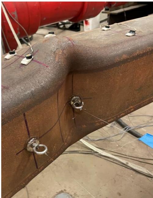
Moderate cupping in plastic hinge region: cycle 23
