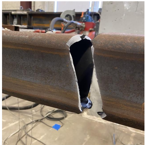
Specimen fractured in tension during first 5.75" cycle
