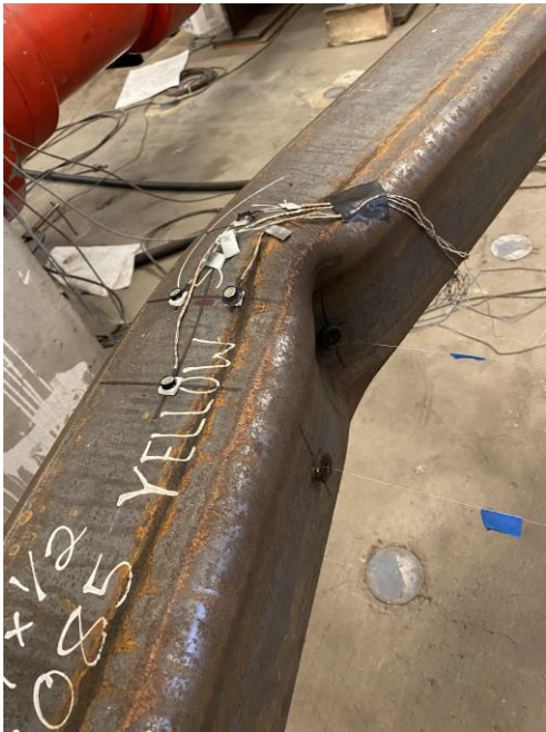
Cupping at Center of Specimen: 3.75" Cycles 1 & 2 C
