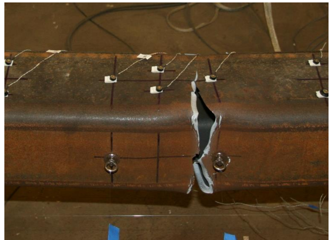
Tearing at the center of the specimen: cycle 23
