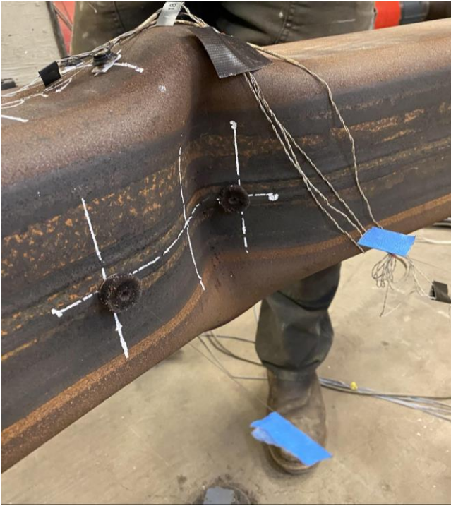
Cupping at Center of Specimen: 2.75" Cycles 1 & 2 C
