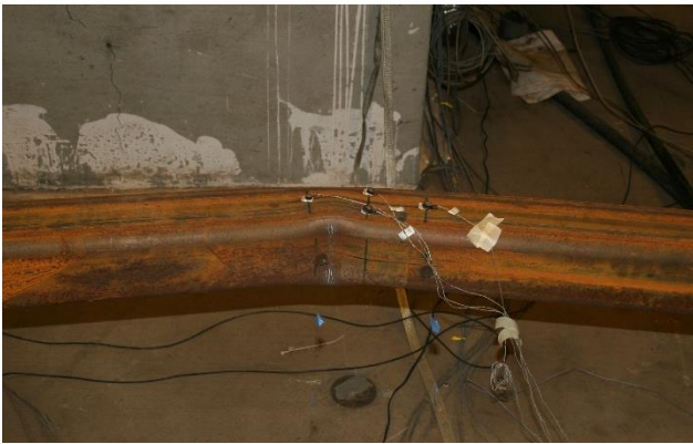
Tearing beginning to develop at center of brace: 5.75" cycles
