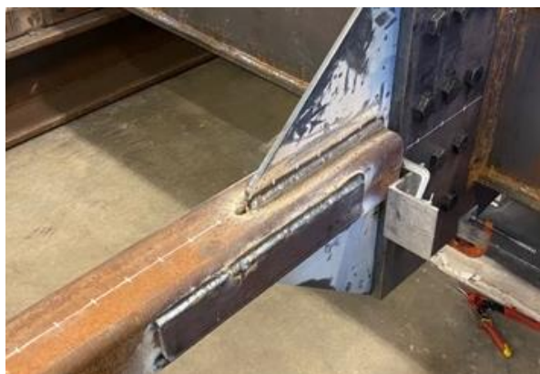
Figure 3.20 Net Section Reinforcement at End Connection
