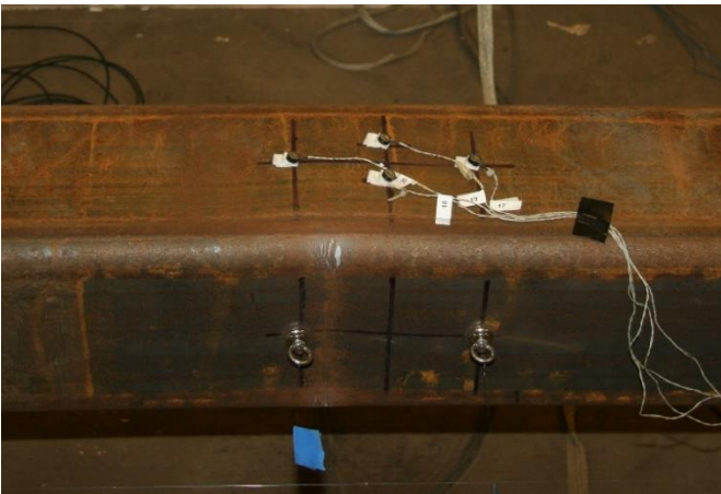
Striations/tearing initiating at the corners: 2.25" T1
