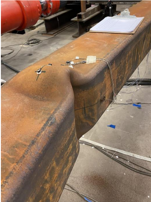
Cupping after Initial Tearing at Corners: 1.75" Cycle 2 C
