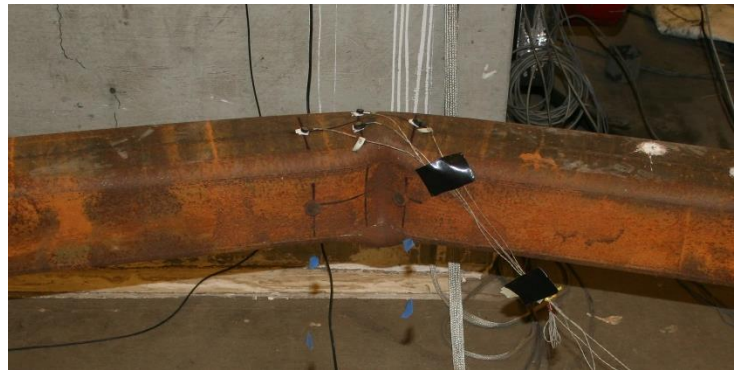
Moderate cupping at center of brace: 3.75" cycles
