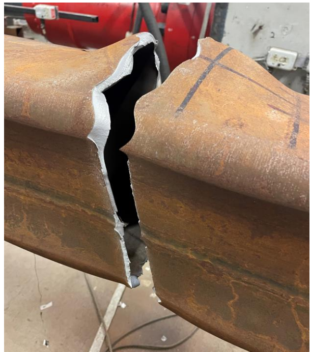
Specimen fractured at first 3.75" tension cycle
