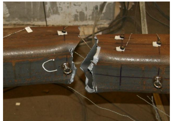
Brace fractured in tension at cycle 34
