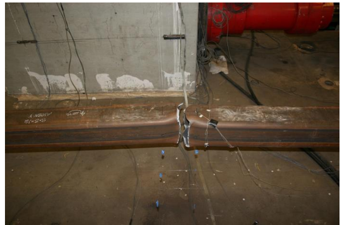
Fractured Specimen: 3.75 Cycle 1 T
