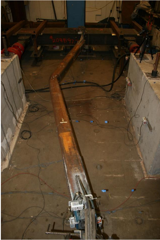
Maximum out of plane displacement: 3.25" C1
