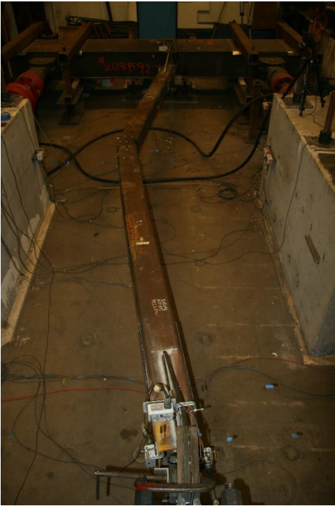
Max out of plane displacement: cycle 19.5
