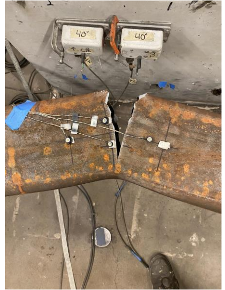
Tearing at Center of Specimen: 3.25" Cycle 1 C
