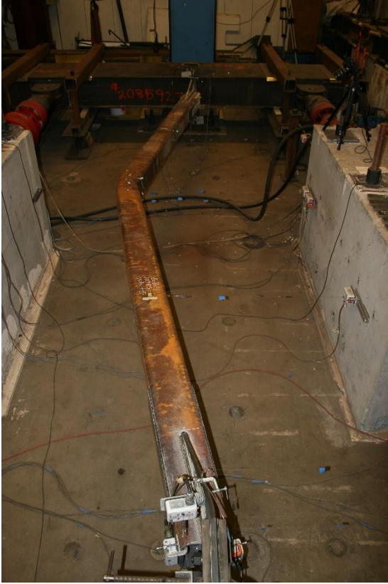
Max out of plane displacement: 3.25" C2
