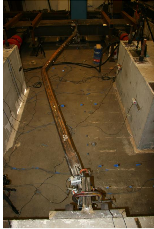
Peak out of plane displacement: 5.25" cycles
