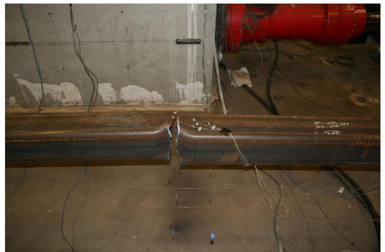
Fractured Specimen during 2.75" Cycle 1 T
