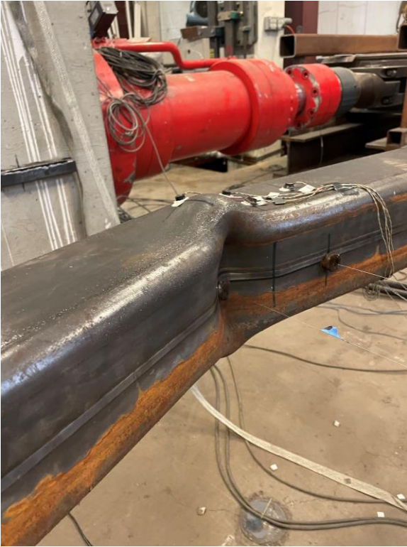
Moderate cupping at center of brace: 3.25" cycles
