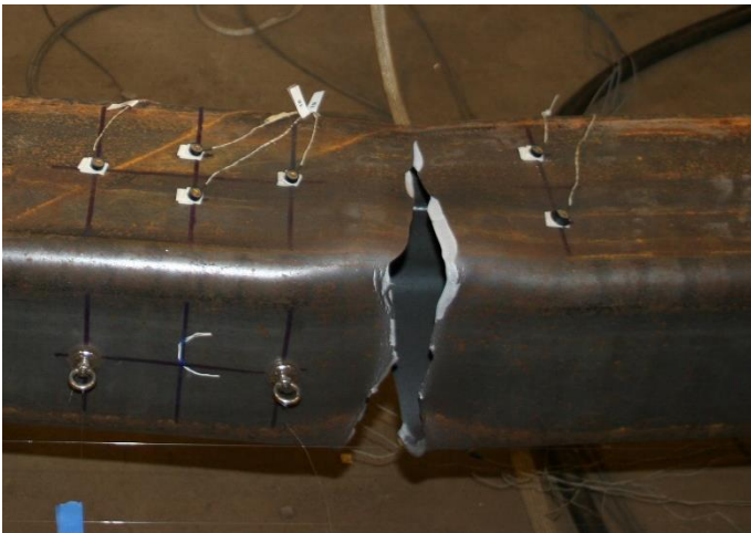
Development of tearing across the brace section: cycle 21
