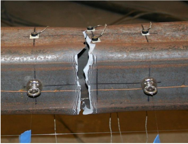
Specimen tore thru east, bottom, and top walls: cycle 28
