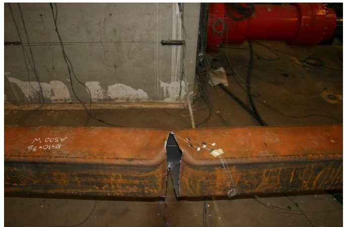
Specimen Immediately Before Fracture: 2.75" Cycle 1 T
