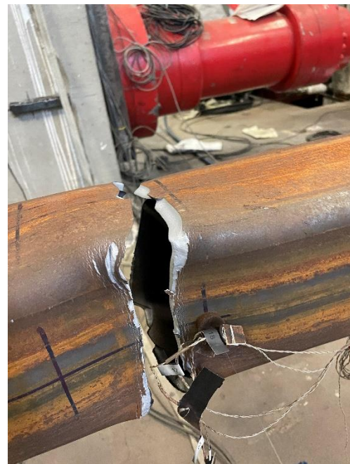
Specimen fractured in tension during first 4.25" cycle
