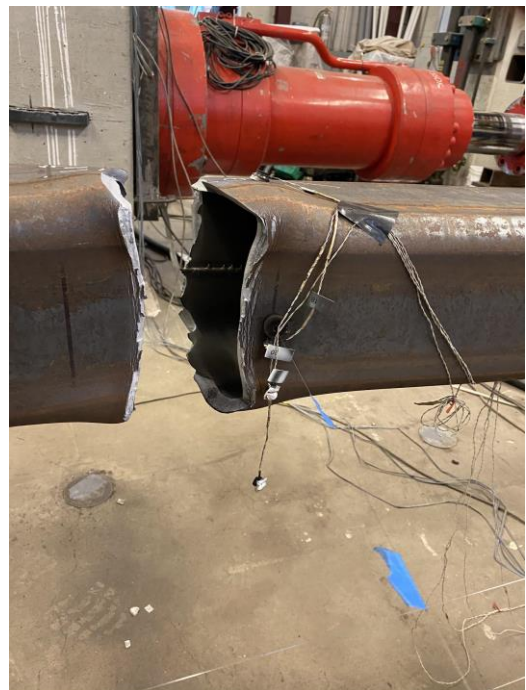
Fractured Specimen after 4.25" Displacement - Cycle 2 T
