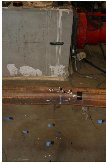
Initiation of Brace Tearing: 4.25” Cycle 2
