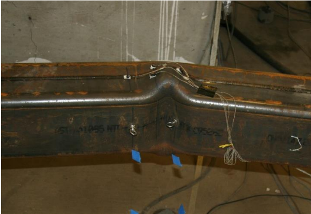
Cupping at the center of the brace: 2.25" cycles
