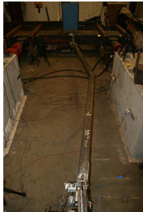
Specimen buckling westward: 4.75" cycle 1
