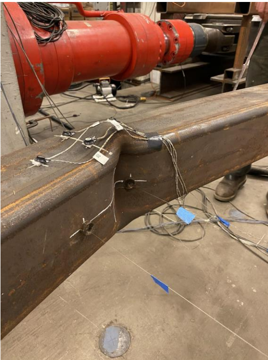
Cupping at Center of Specimen: 3.25" Cycle 1 C
