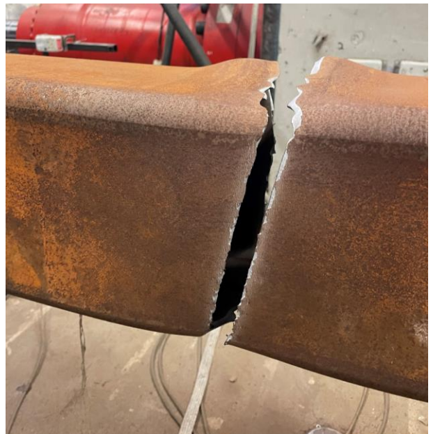
Specimen fractured at first cycle of 2.75" disp.
