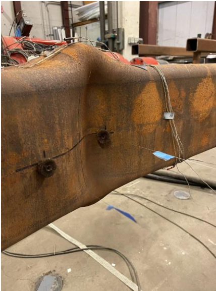
Cupping at Center of Specimen: 1.75" Cycle 1 C
