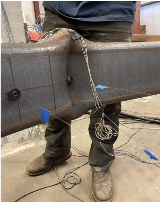
Cupping at Center of Specimen: 2.75" Cycle 1 C
