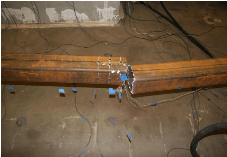
Peak Out of Plane Displacement (West): 3.25" Cycle 1
