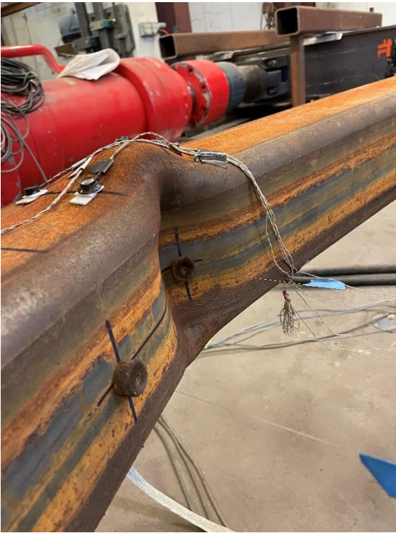
Moderate cupping at center of brace: 4.25" cycles
