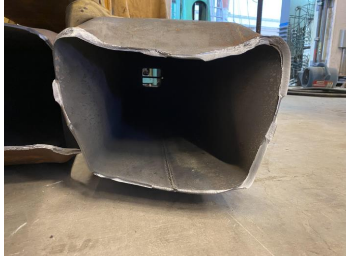
Cross Section of Fractured Specimen After Testing
