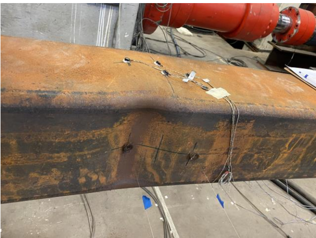
Cupping at Center of Specimen: 1.25" Cycle 1 C
