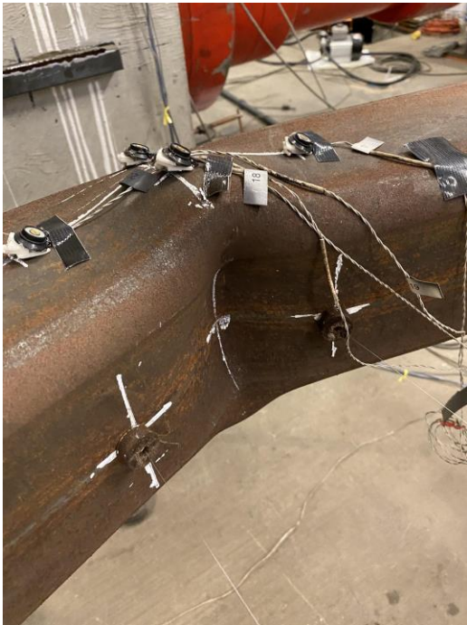
Cupping at Center of Specimen: 4.75" Cycles
