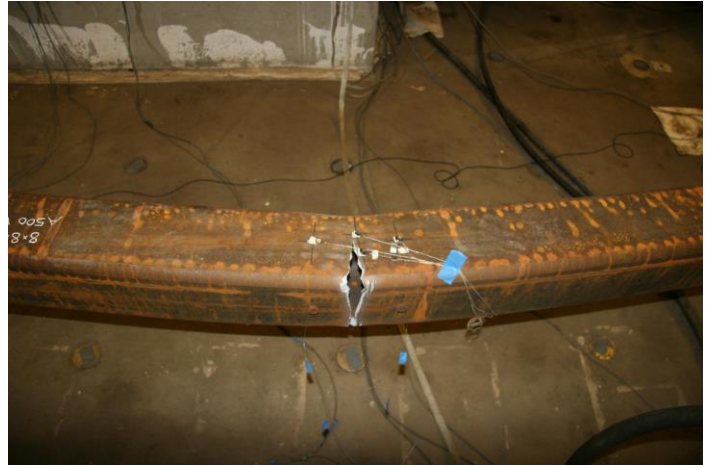
Initiation of Striations and Tearing: 3.25" Cycle 1 T
