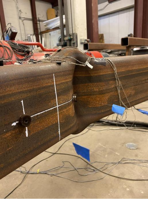
Cupping at Center of Specimen: 2.25" Cycles 1 and 2 C
