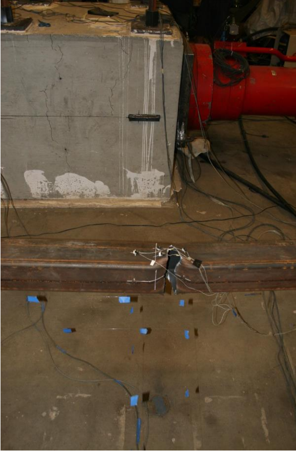
Tearing Prior to Fracture: 3.75" Cycle 1 T
