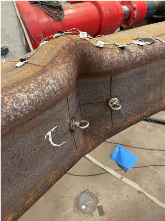
Major cupping prior to tearing: 2.75" cycles
