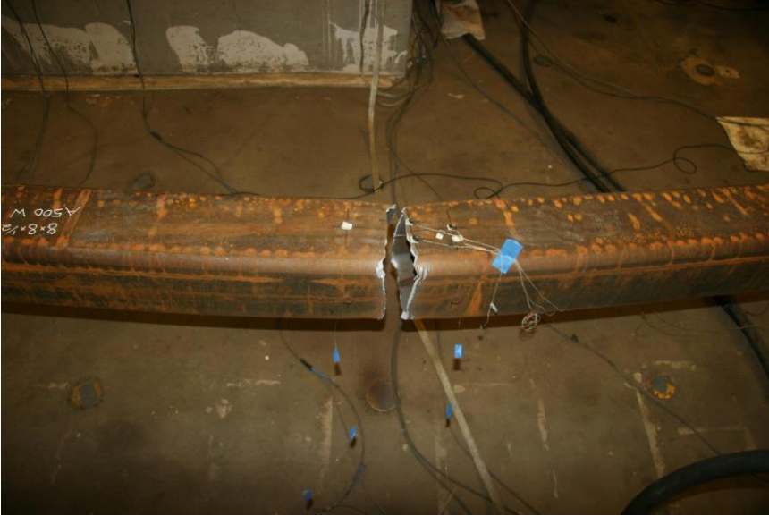
Fractured Specimen: 3.25" Cycle 1 T
