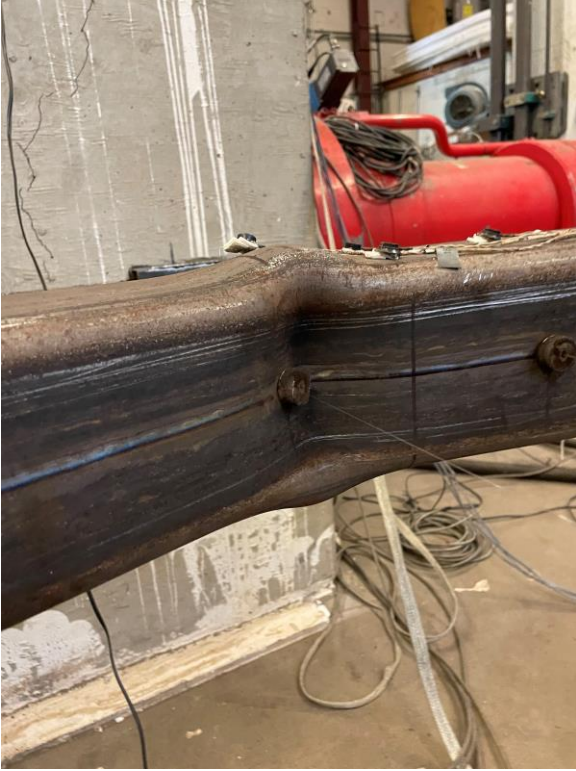
Moderate cupping at center of brace: 4.75" cycles
