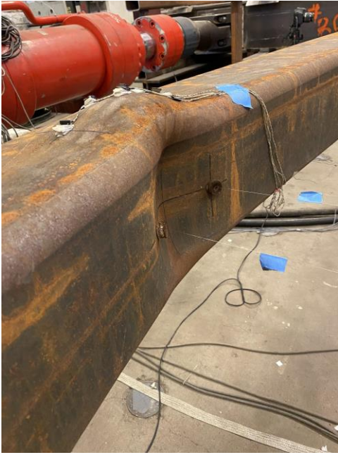
Cupping at Center of Specimen: 2.25" Cycle 2 C
