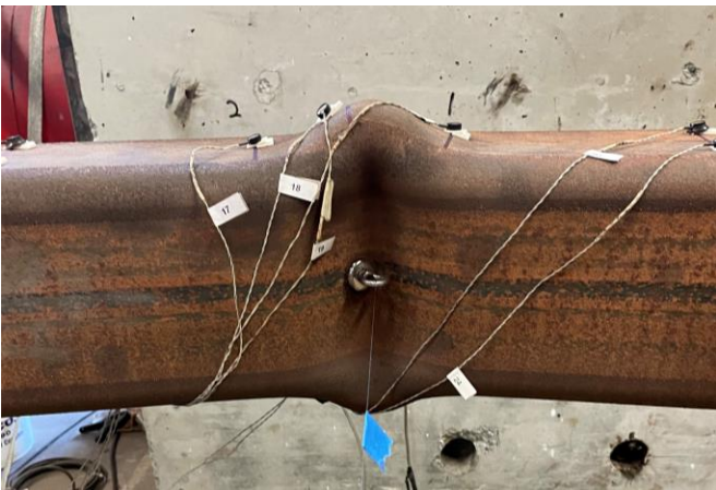
Severe cupping at the center of the specimen: cycle 21.5
