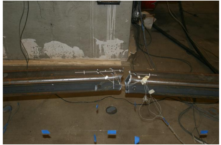
Brace Fracture: 2nd Cycle at 5.75"
