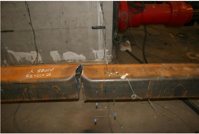
Fractured Specimen: 3.75 Cycle 1 T
