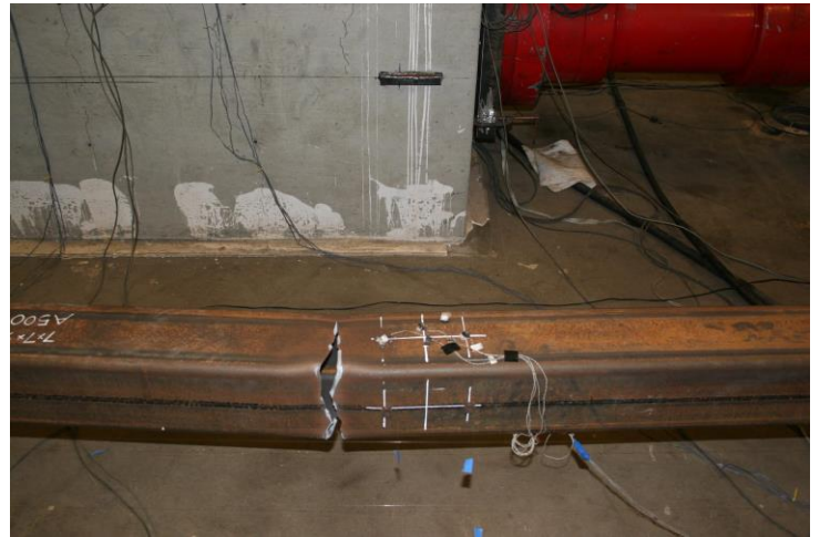
Tearing at Center of Specimen: 2.25" Cycle 1 T
