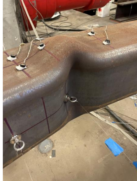
Major cupping during final compression cycle prior to fracture
