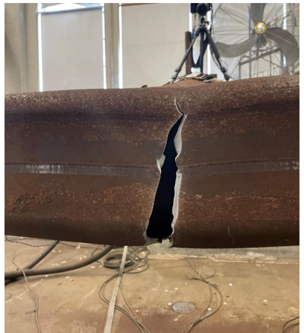
Tearing thru west wall while buckling: 3.25" C1
