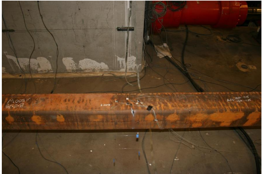
Initiation of Striations and Tearing: 1.75" Cycle 2 T
