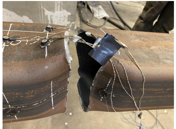
Fractured Specimen after 3.25" Displacement - Cycle 1 T
