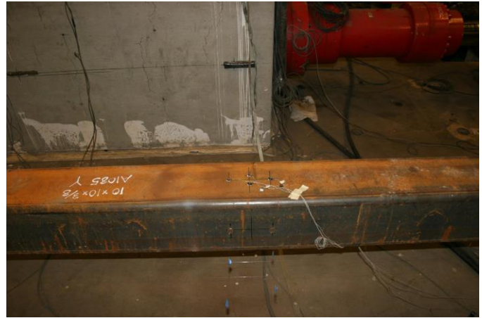
Development of Striations at Corners: 1.75" Cycle 1 T
