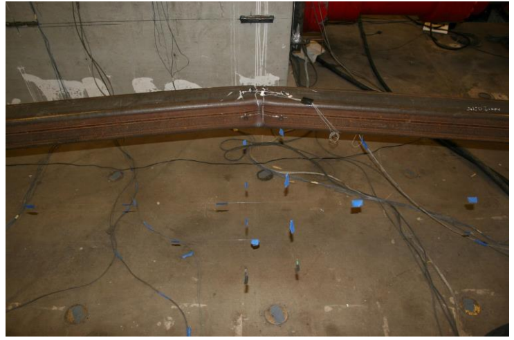
Ductile Fracture of Specimen in Compression at 3.75"
