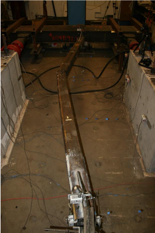
Maximum out of plane displacement: Cycle 20 Cycle 20
