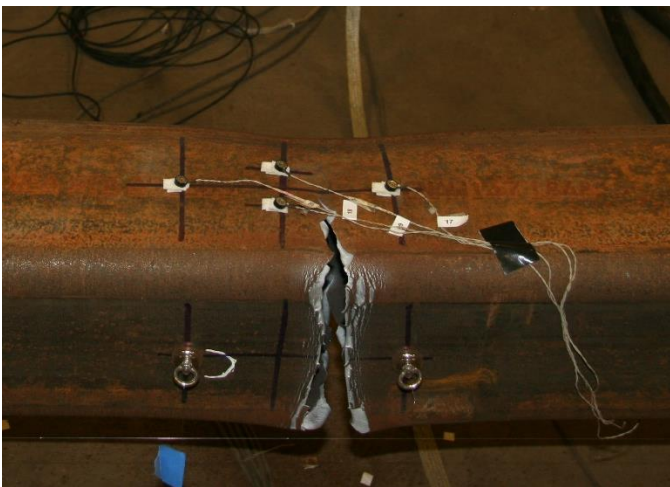
Specimen tearing halfway thru cross-section: 3.25" T1
