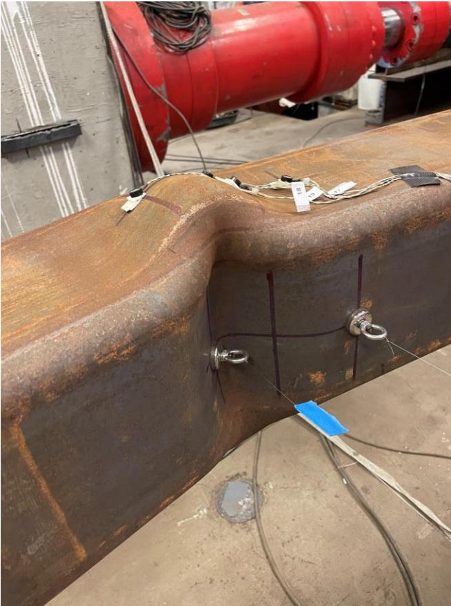
Severe cupping at center of specimen: 2.25" C2
