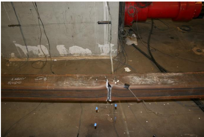
Tearing at Center of Specimen: 3.25" Cycle 1 T
