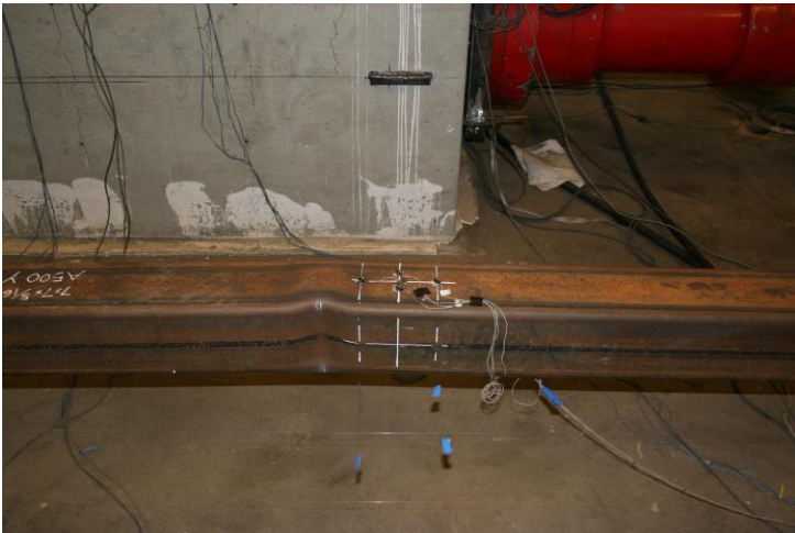
Initial Striations at Center of Specimen: 2.25" Cycle 1 T
