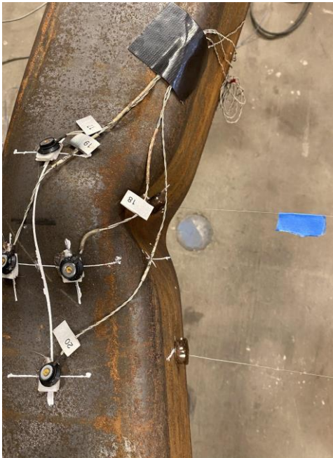
Cupping at Center of Specimen: 3.75" Cycle
