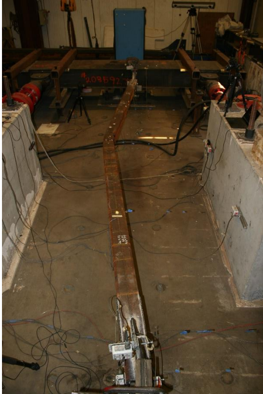
Fracture as brace buckled in compression: 4.25" cycles
