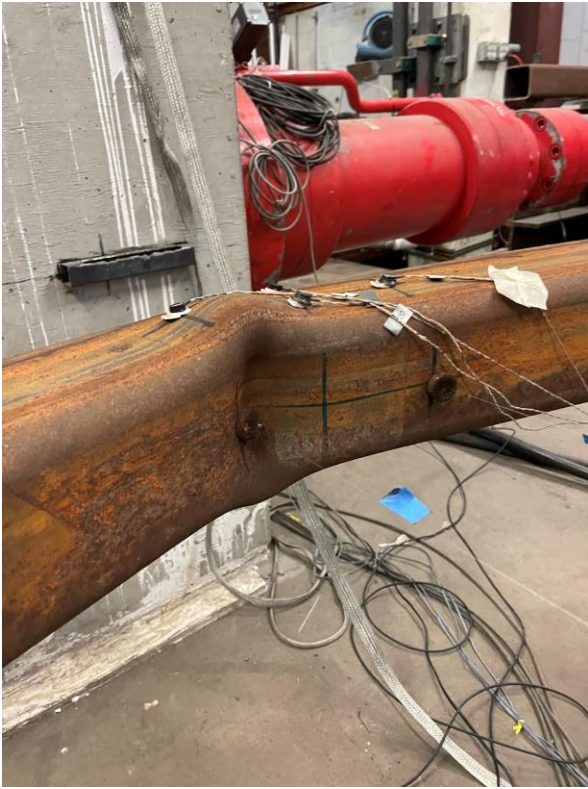
Moderate cupping at center of brace: 5.25" cycles
