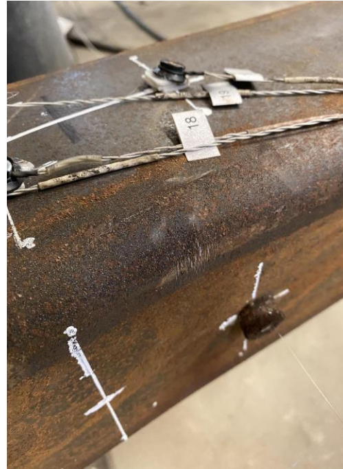
Initial Striations at Center of Specimen: 2nd Cycle at 3.75"
