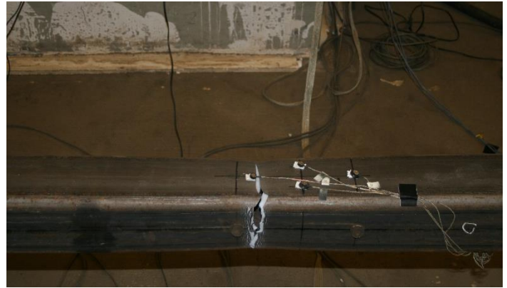
Tearing thru three walls: 4.75" cycles
