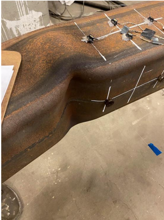
Cupping at Center of Specimen: 1.75" Cycle 1 & 2 C
