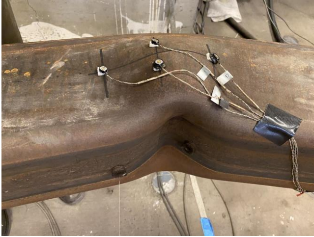
Cupping at Center of Specimen: 3.25" Cycles 1 & 2
