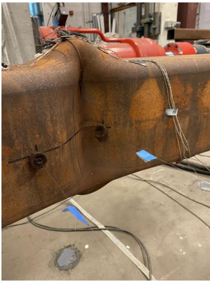
Cupping after Initial Tearing: 1.75" Cycle 2 C
