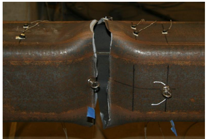
Tearing opening at incipient fracture: cycle 19
