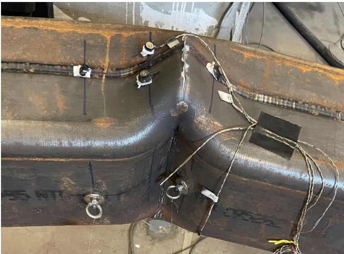
Cupping at the center after tearing: 2.25" cycle 2
