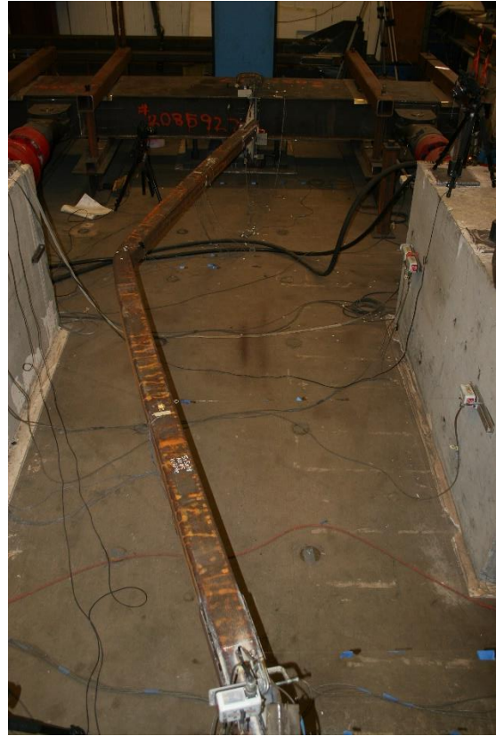
Peak out of plane displacement: 5.25" cycles
