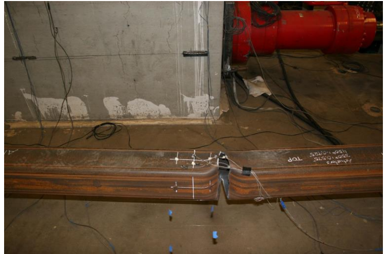
Tearing Through Specimen: 2.25" Cycle 2 T
