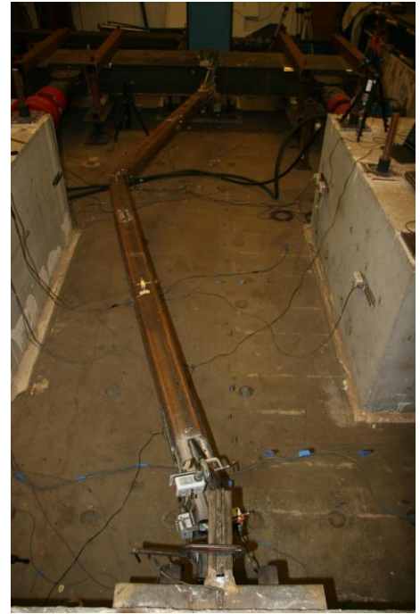
Peak Out of Plane Displacement: 5.25" Cycle
