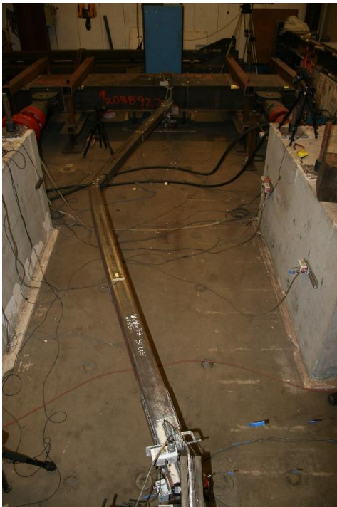
Specimen buckling eastward after tearing: 4.75" cycle 2
