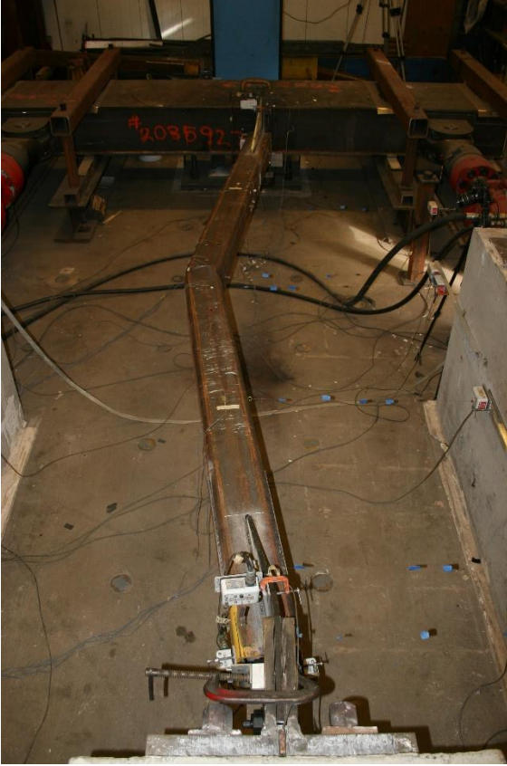
Maximum out of plane displacement: cycle 18
