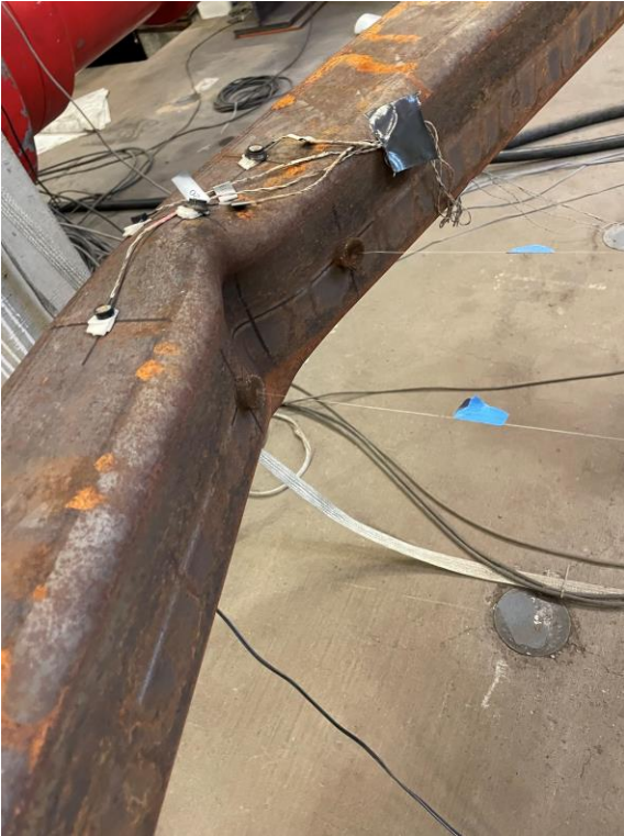
Moderate cupping at center of brace: 5.25" cycles
