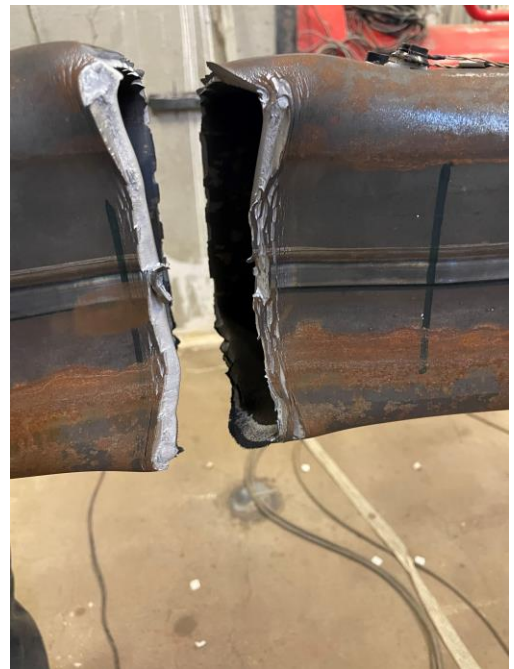
Specimen fractured in tension during first 3.75" cycle
