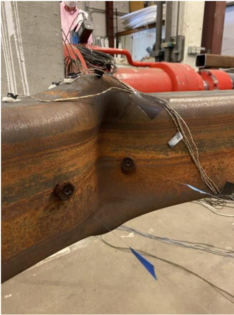
Cupping at Center of Brace: 3.75” Cycles
