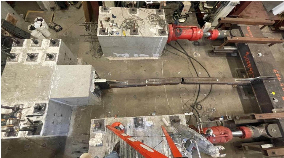
Figure 3.4 Configuration of Test Frame for 183.5" Brace Specimen
