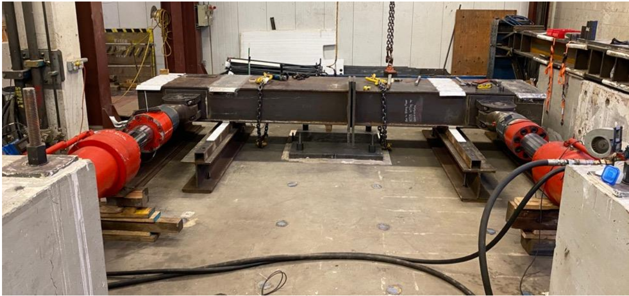
Figure 3.7. Orientation of Actuators and Sliding Beam
