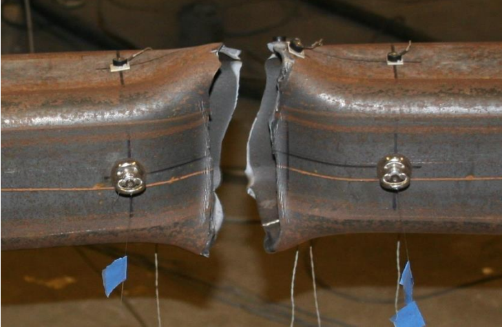
Fracture at the center of the brace: cycle 29
