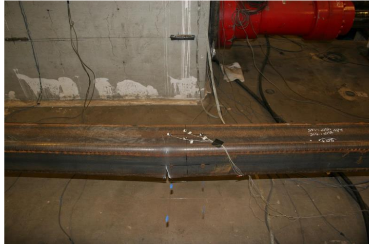
Development of Striations and Tearing: 2.25" Cycle 2 T
