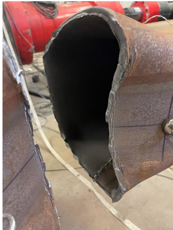
Fracture at the center of the specimen: 3.75" T1
