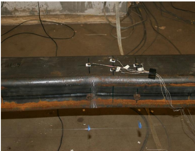
Striations develop at center of brace: 3.25" cycles
