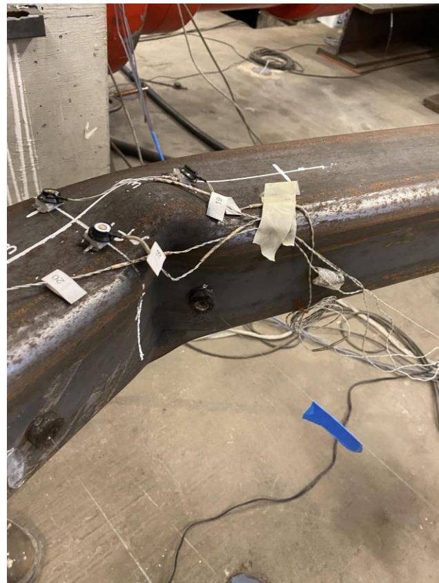
Cupping at Center of Specimen: 5.25" Cycles
