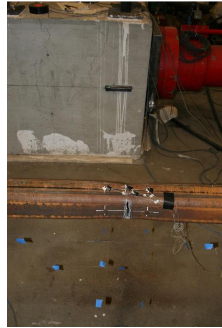
Brace Tearing: 4.75” Cycle 1
