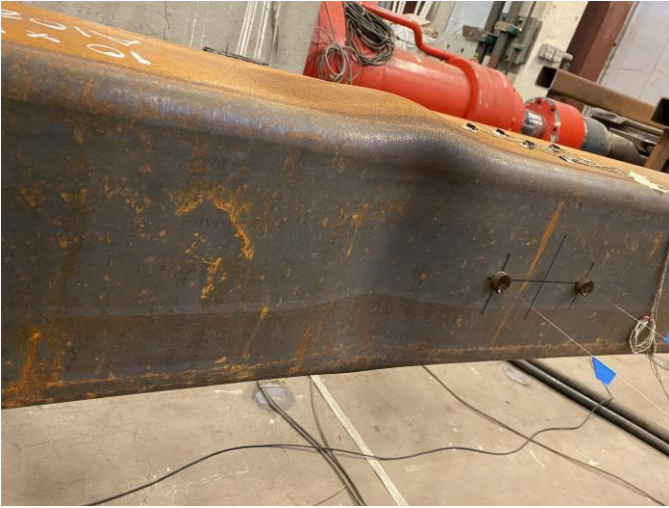
Cupping at Center of Specimen: 1.25" Cycle 1 C
