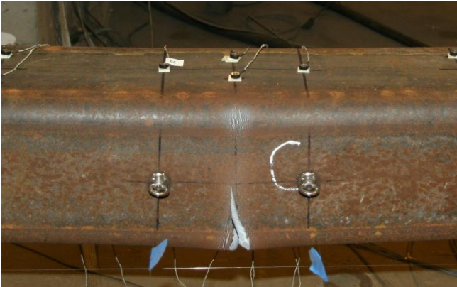
Initial tearing on east wall: cycle 17
