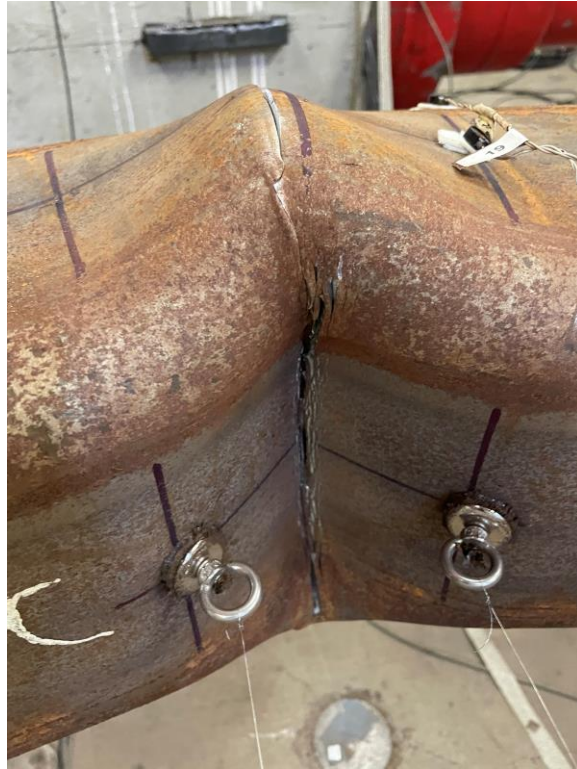
Cupping after specimen tore halfway thru: 3.25" cycles
