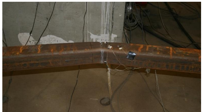
Fracture thru west wall in compression: 5.25" cycles
