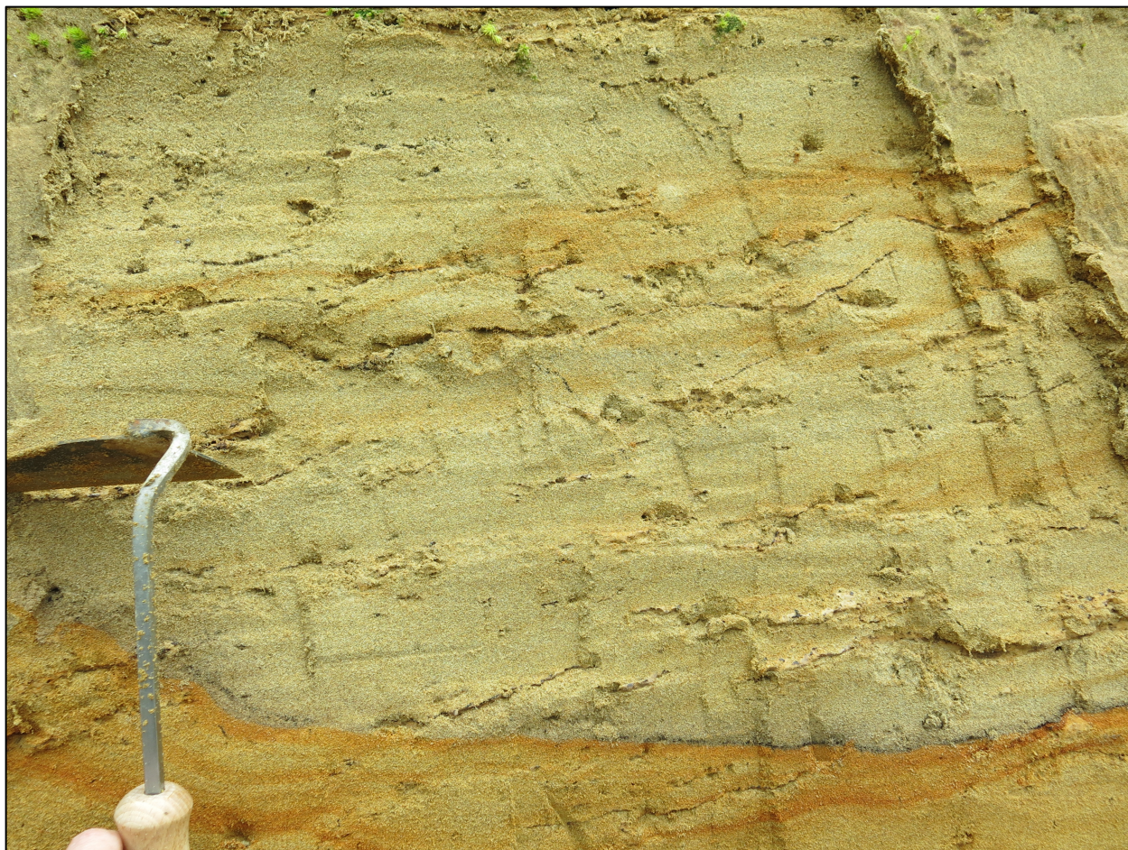
Figure 8 Subangular to subrounded, fine quartz-rich sand with minor lithics, thinly bedded with minor cross bedding. Oxidized and with minor interbeds of silts. These are field station 19GW89.1 and 20GW0701.1. Unit Qss. View to the east-northeast.
