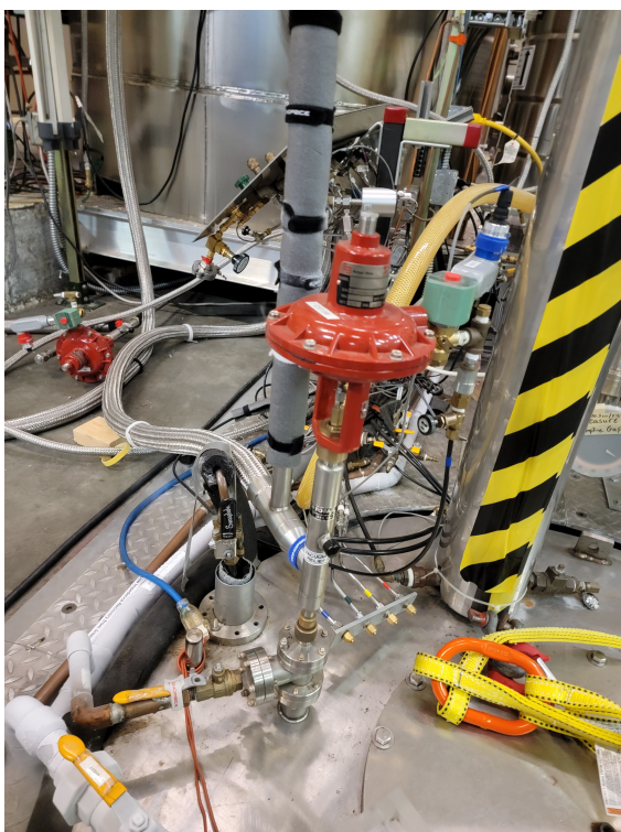
Figure 4.20: An electronic liquid helium fill pump. 4 of these pumps allow for automated fills of the magnet cryostat and its reservoir from the mother dewar.
