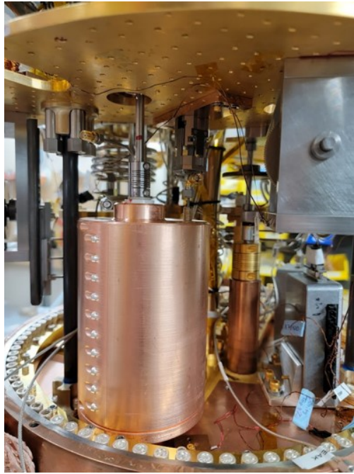
Figure 9.14: The run 1D Sidecar cavity installed in the ADMX insert with piezoelectric motors mounted.
