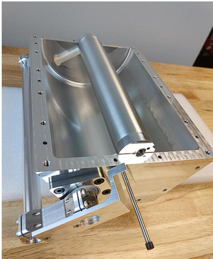
Figure 6.15: An open aluminum reduced length EFR prototype cavity being tested at LLNL.
