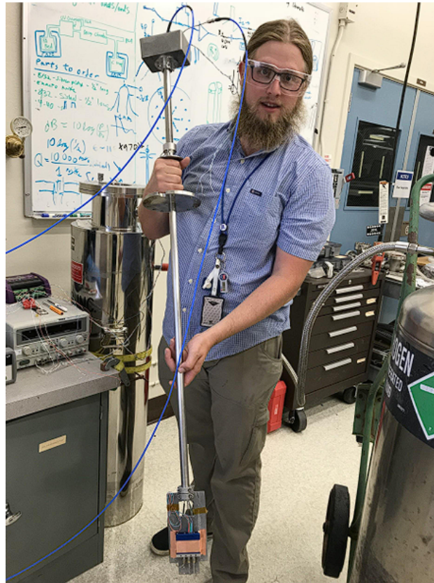
Figure 4.17: The author holding the coaxial switch mounted to paddle for cryogenic testing. The cryogenic vessel located behind.
