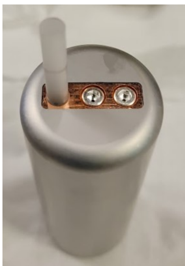
Figure 9.11: The Sidecar tuning rod with copper axle tab installed. The sapphire axle was epoxied to the copper tab with stycast. Vented, silver-plated 8-32 screws attached the tab to the Nb-substrate tuning rod.
