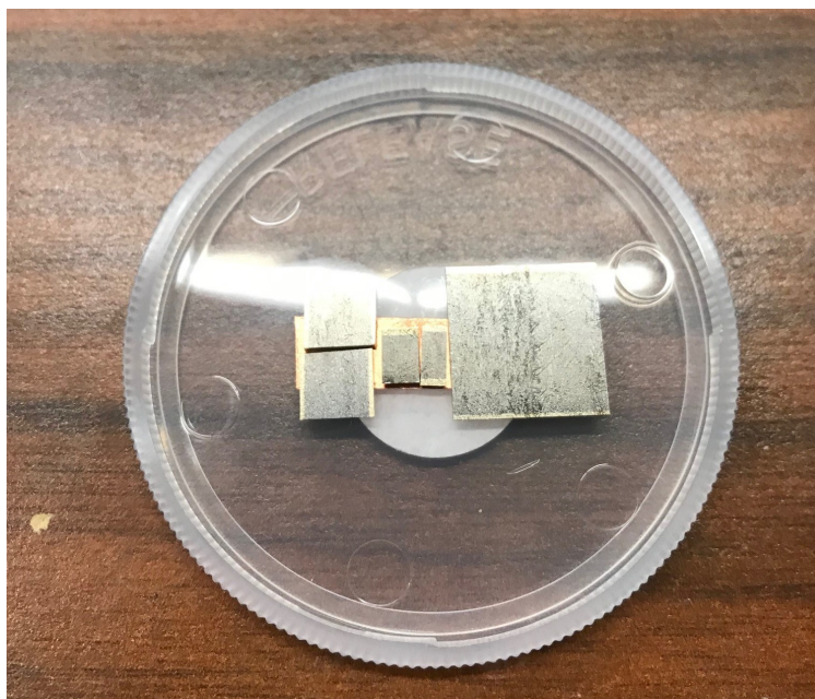
Figure 8.12: Nb 3 Sn coating deposited on bronze substrate. This deposition work was done at Florida State University by Lance Cooley's group, see Ref. [121] for details.
