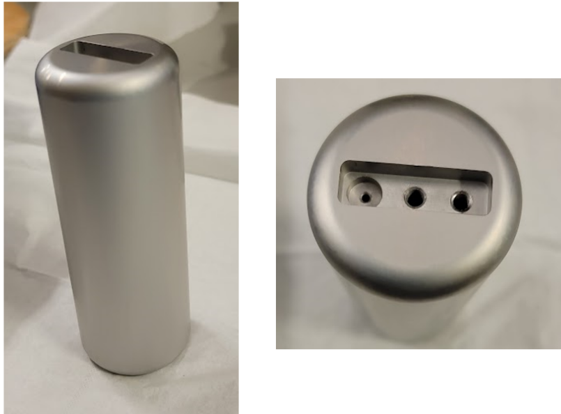
Figure 9.5: The \text{Nb}_3\text{Sn} coated tuning rod from a side and top viewpoint. The rod is 1.75" in diameter, and features an inset for mounting the copper sapphire axle tabs. The center and right holes are tapped with 8-32 threads for mounting these tabs. The center hole goes through the length of the rod so that it could be hung by a wire in the coating furnace.
