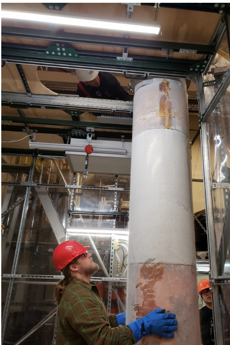
Figure 4.5: Mounting ADMX insert to clean room ceiling after run 1B.
