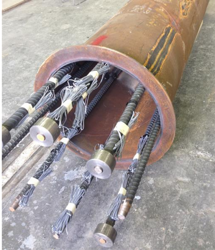
Figure 4.11: Specimen WRC annular ring and reinforcing bars
