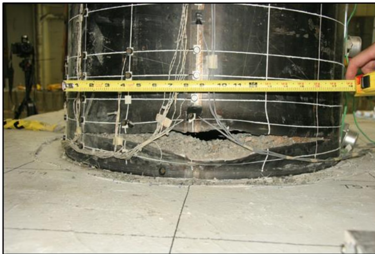
Figure 5.71: EMB96 South tear propagation at 9.15% drift North
