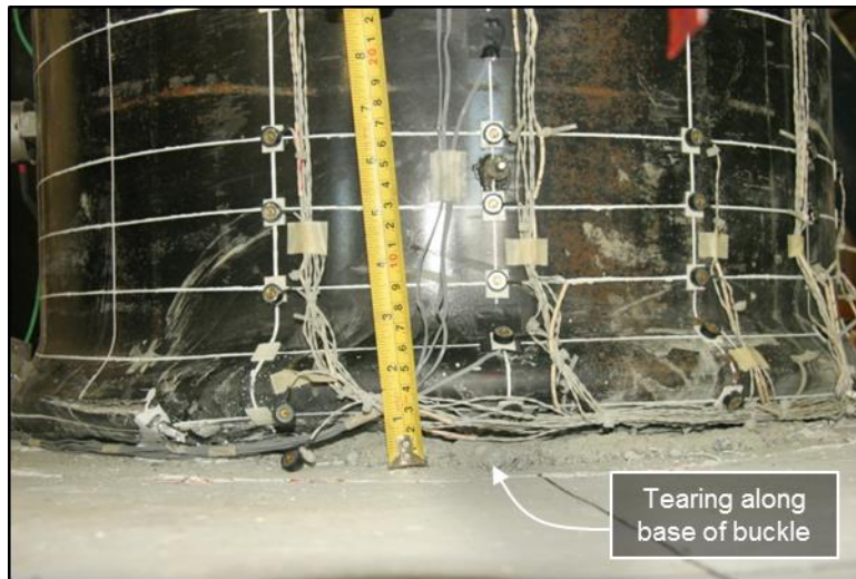
Figure 5.72: EMB96 North tear propagation during second cycle at 8.60% drift South
