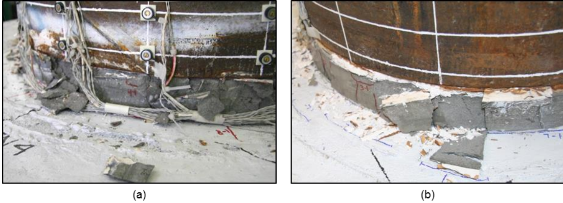
Figure 5.54: WRC Soffit crushing (a) North side of specimen, (b) South side of specimen
