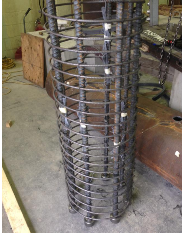
Figure 4.13: Reinforcing cage of Specimen RC
