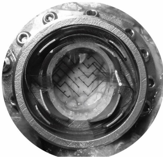
Figure 4.5: Chamber and MMAD implanted prior to cap being placed during surgery. MMAD arms coiled in slots.
