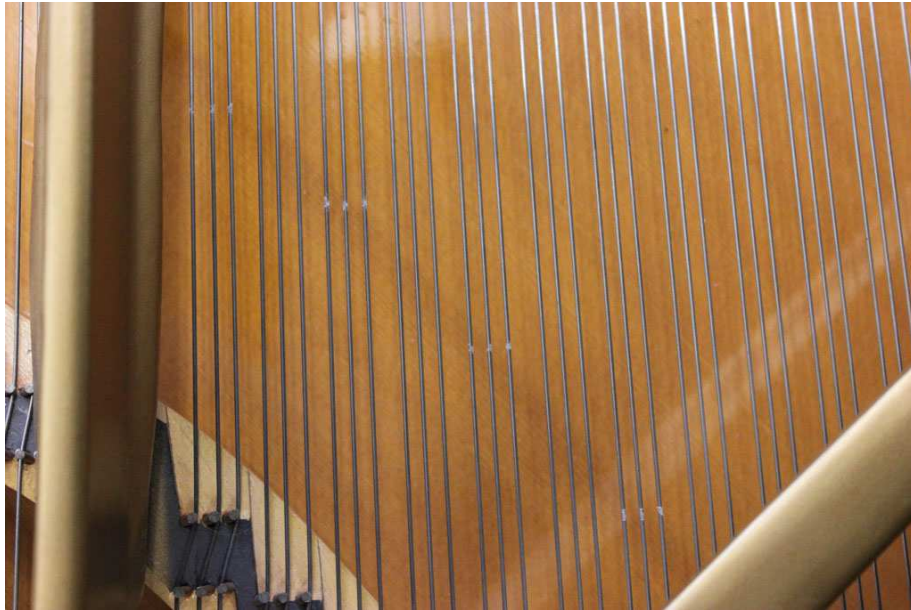
Figure 20: Chalk markings for the 2nd harmonic
