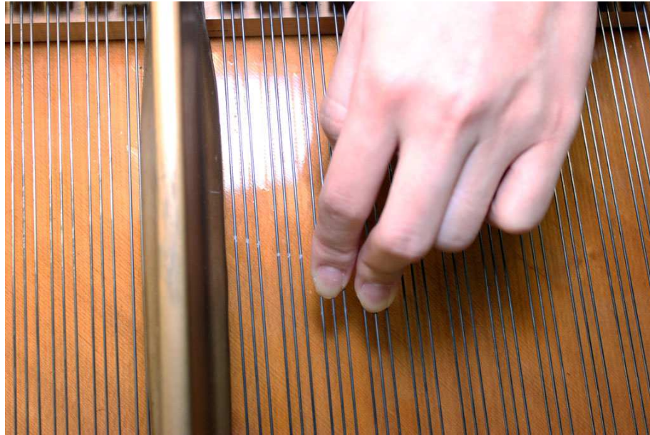
Figure 21: Pressing on strings for the 2nd harmonic
