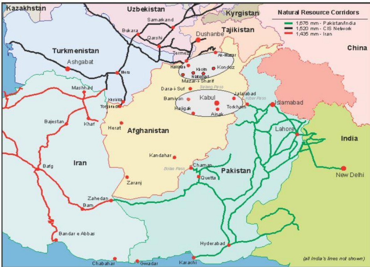
Figure 3. 1 This map shows all of the rail lines in the region according to track gauge. Each region uses a different gauge from one another and are therefore incompatible and require a “break of gauge” to travel trains between tracks of different gauge width.
