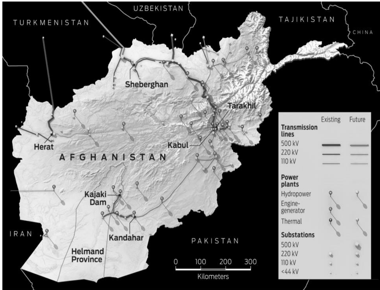
Figure 1. Map showing location and extent of separate power grid systems, as well as power plants and substations. ( Zorpette, 2011).
