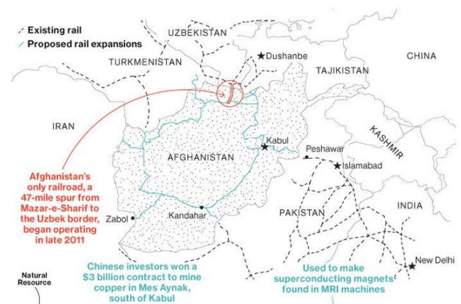
Figure 2. The only rail line in Afghanistan in red and the proposed "Rail Ring" in blue that connects to rail networks in neighboring countries.
