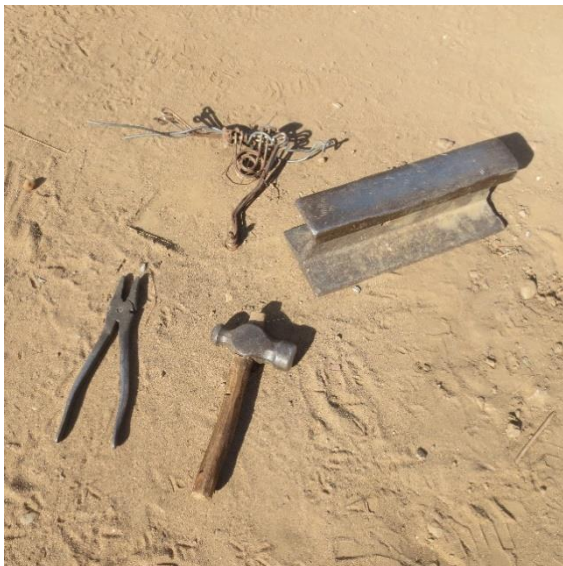
Figure 19. Enoch Nyazvigo’s tools for building mbira, including a special kind of small hammer, wire, pliers, and a piece of railroad track for pounding and shaping keys.
