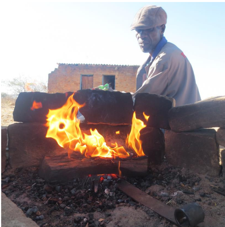
Figure 11. Sekuru Matomati heating the fire by pumping the bellows. He does this to heat the long piece of metal that sits under the fire before pounding it.
