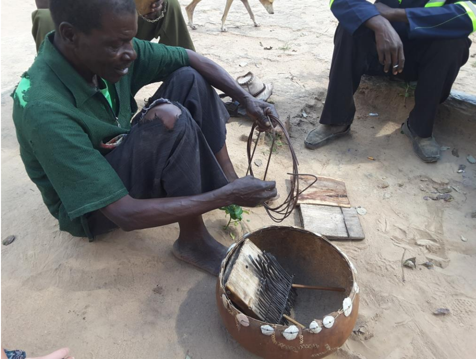
Figure 14. Efraim Masarakufa holding up the type of wire he uses to pound keys. Masarakufa's madhebhe is shown in the resonator alongside two unfinished madhebhe. May 2017.
