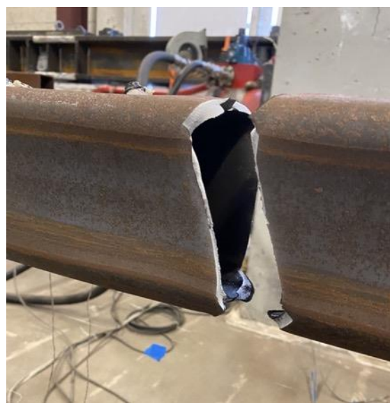
Peak out of plane displacement: 5.25" cycles
