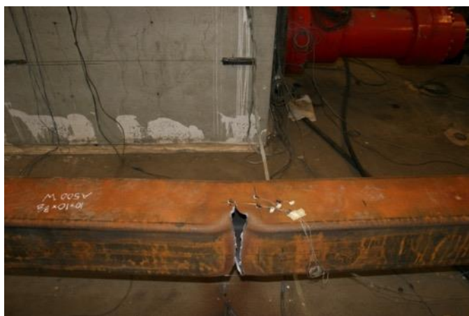
Propagation of Tearing at Center: 2.25" Cycle 1 T
