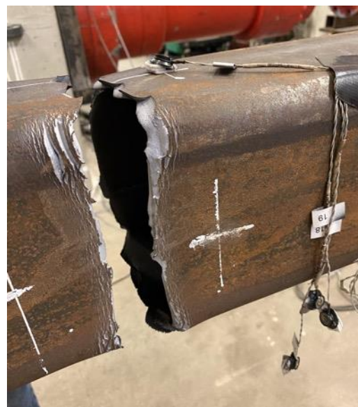
Fractured Specimen: First Cycle at 4.25"
