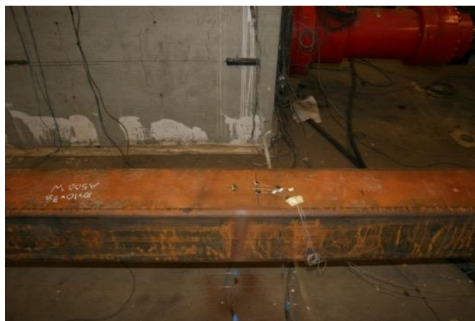
Initiation of Striations and Tearing: 1.75" Cycle 1 T
