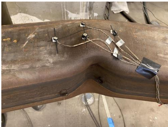
Cupping at Center of Specimen: 3.25'' Cycles 1 &amp; 2
