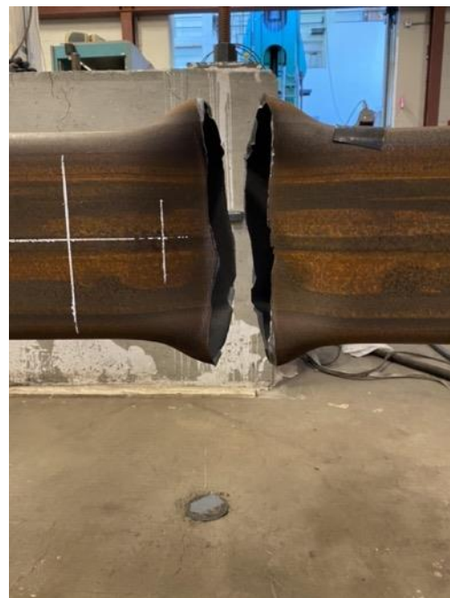
Fractured Specimen: 2.75" Cycle 1 T
