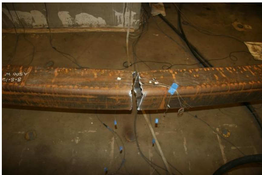
Fractured Specimen: 3.25" Cycle 1 T
