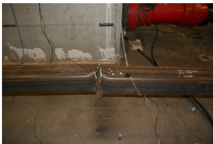
Fractured Specimen during 2.75" Cycle 1 T
