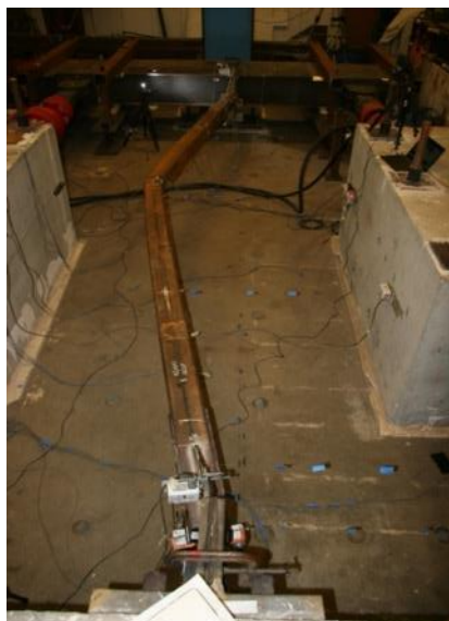
Peak Out of Plane Displacement (West): 3.25" Cycle 1
