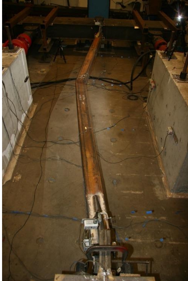
Peak Out of Plane Displacement: 1.75" Cycle 1 & 2
