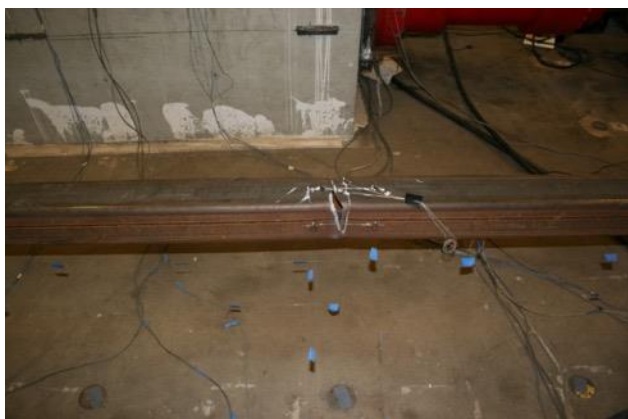
Tearing at Center of Specimen: First Cycle at 3.75"
