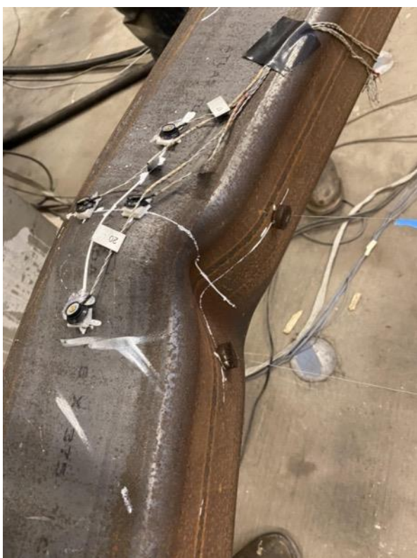
Cupping at Center of Specimen: 3.75" Cycle 1
