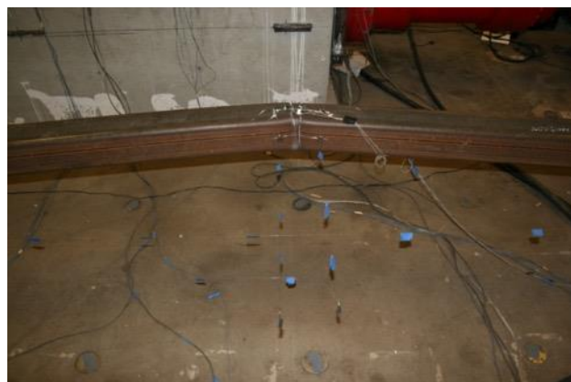
Ductile Fracture of Specimen in Compression at 3.75"
