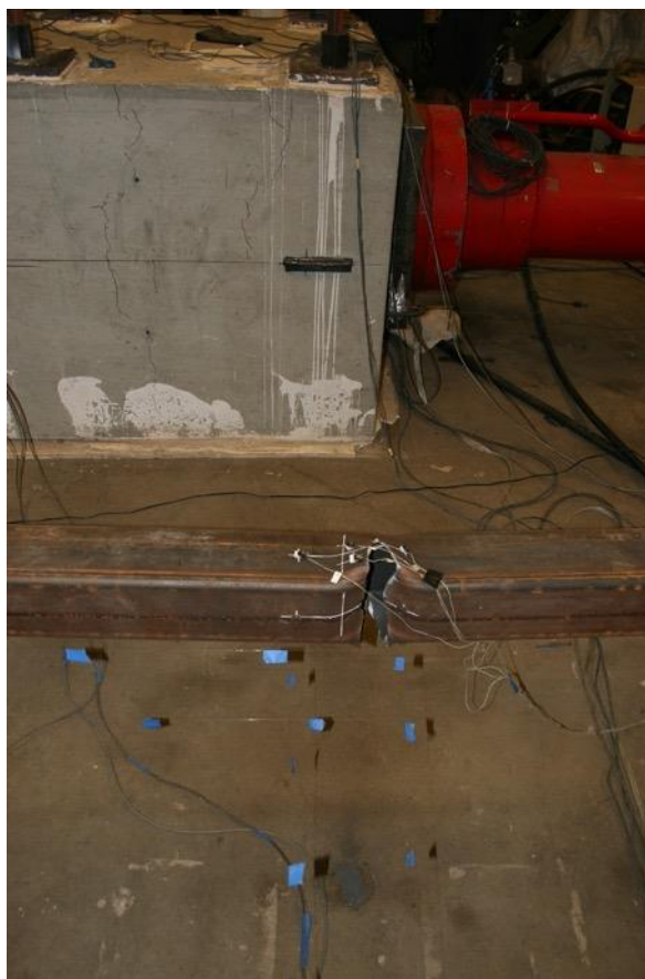
Tearing Prior to Fracture: 3.75" Cycle 1 T
