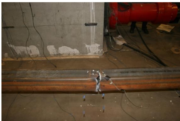
Tearing at Center of Specimen: 4.25” Cycles
