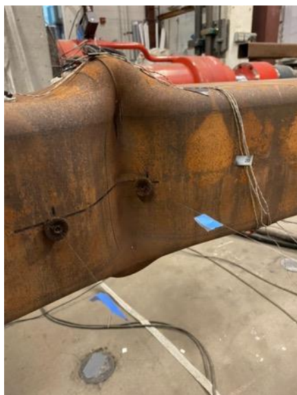
Cupping after Initial Tearing: 1.75" Cycle 2 C
