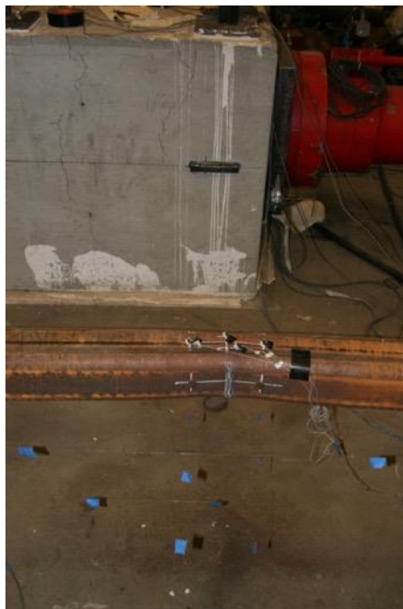
Initiation of Brace Tearing: 4.25" Cycle 2
