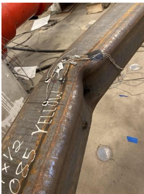
Cupping at Center of Specimen: 3.75" Cycles 1 & 2 C
