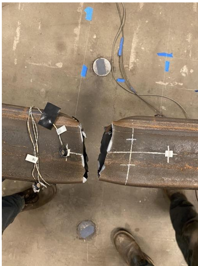
Fractured Specimen: 3.75" Cycle 1 T
