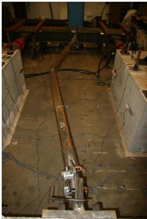
Peak Out of Plane Displacement: 3.75" Cycles
