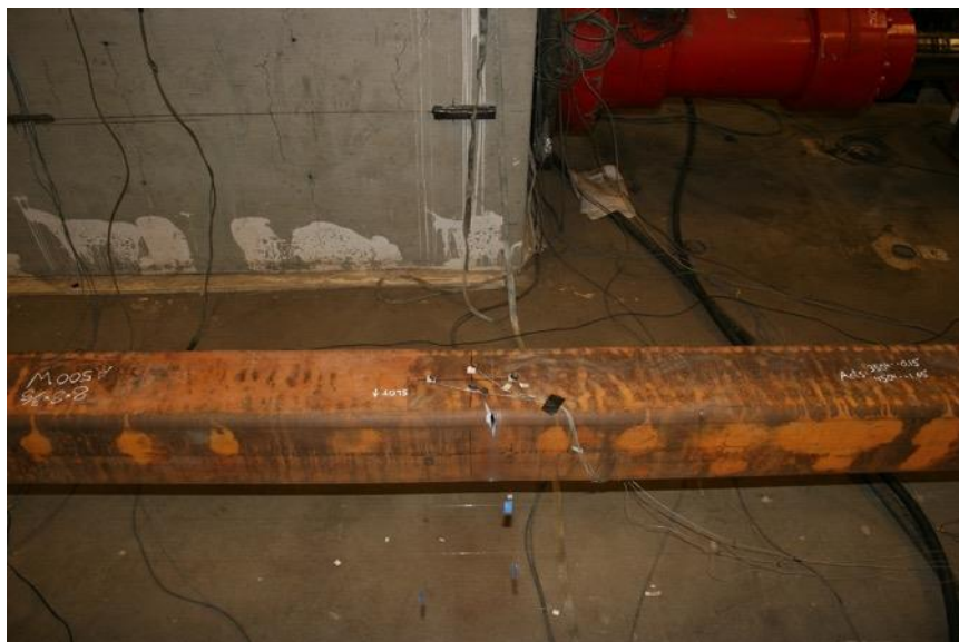
Initiation of Striations and Tearing: 1.75" Cycle 2 T
