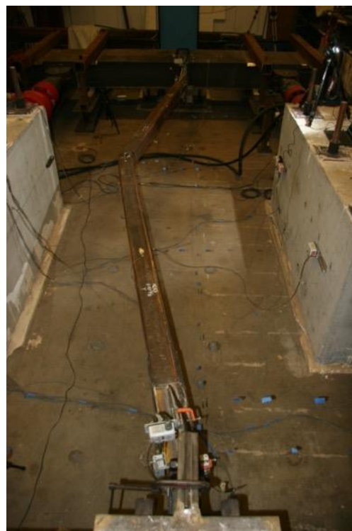
Peak Out of Plane Displacement: 3.25" Cycles
