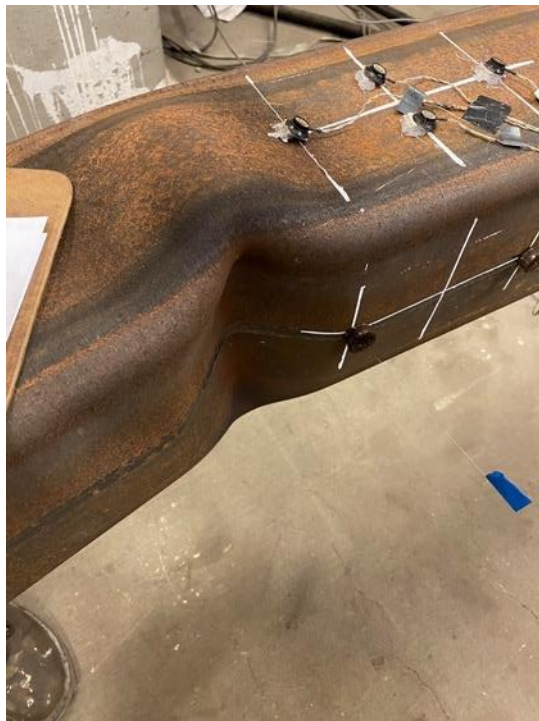
Cupping at Center of Specimen: 1.75" Cycle 1 & 2 C
