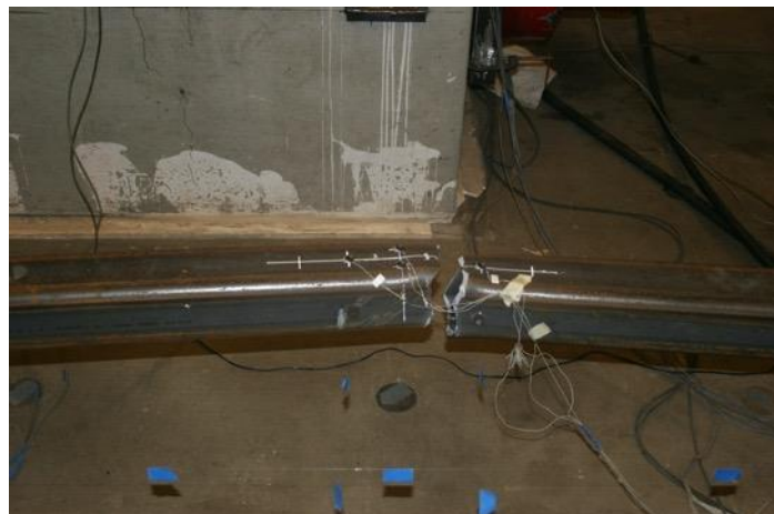
Brace Fracture: 2nd Cycle at 5.75"
