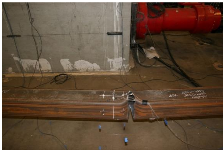
Tearing Through Specimen: 2.25" Cycle 2 T
