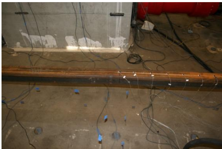
Striations beginning to develop at center of brace: 5.25" cycles
