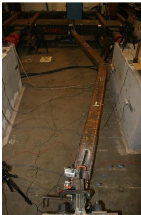
Peak Lateral Displacement: East 3.25" Cycle 1 C
