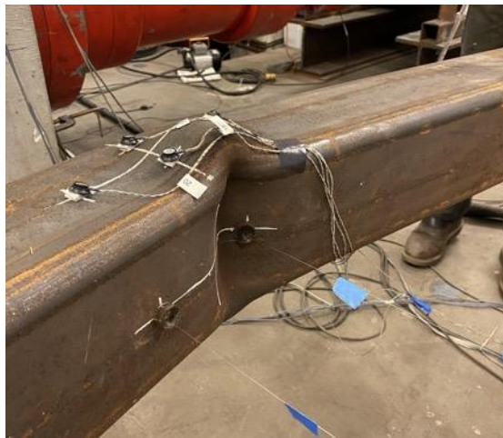
Cupping at Center of Specimen: 3.25" Cycle 1 C
