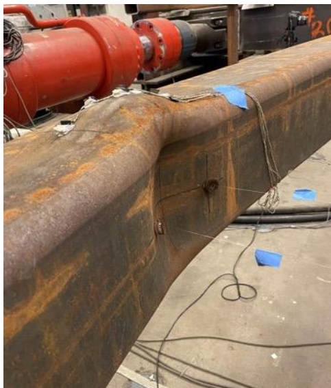
Cupping at Center of Specimen: 2.25" Cycle 2 C
