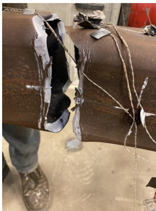
Fractured Specimen: Second Cycle at 5.25"
