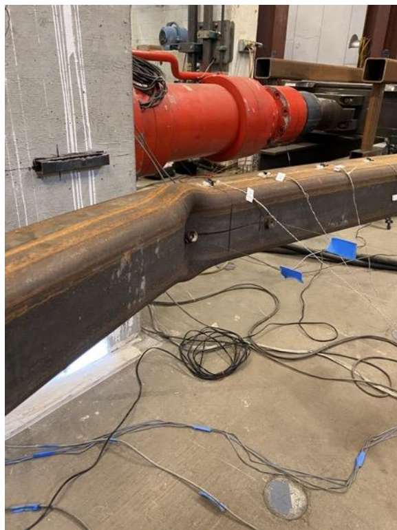
Moderate cupping at center of brace: 5.25" cycles
