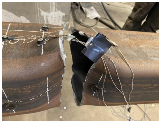
Fractured Specimen after 3.25" Displacement - Cycle 1 T
