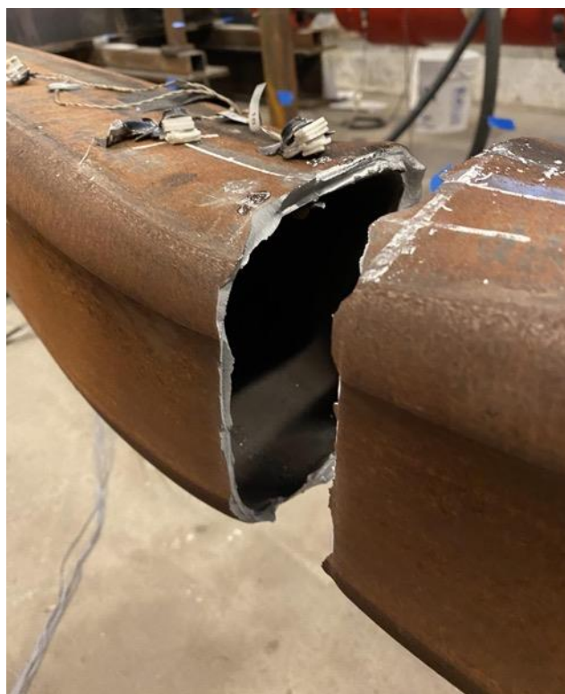
Fractured Specimen: After Cycle 1 at 4.75"
