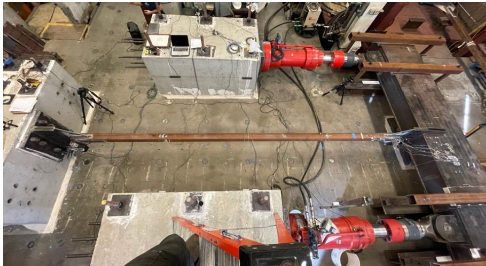
Figure 3.13. Orientation of Test Frame and Specimen on Strong Floor
