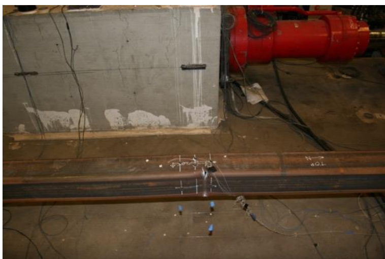
Initiation of Tearing at Center of Specimen: 2.75" Cycle 2 T
