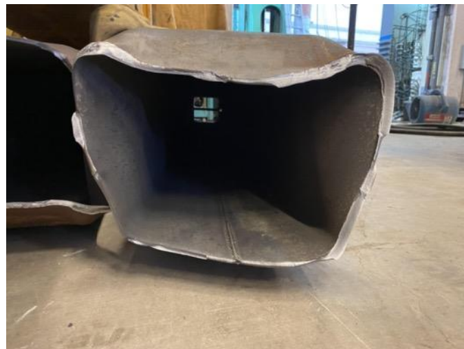
Cross Section of Fractured Specimen After Testing
