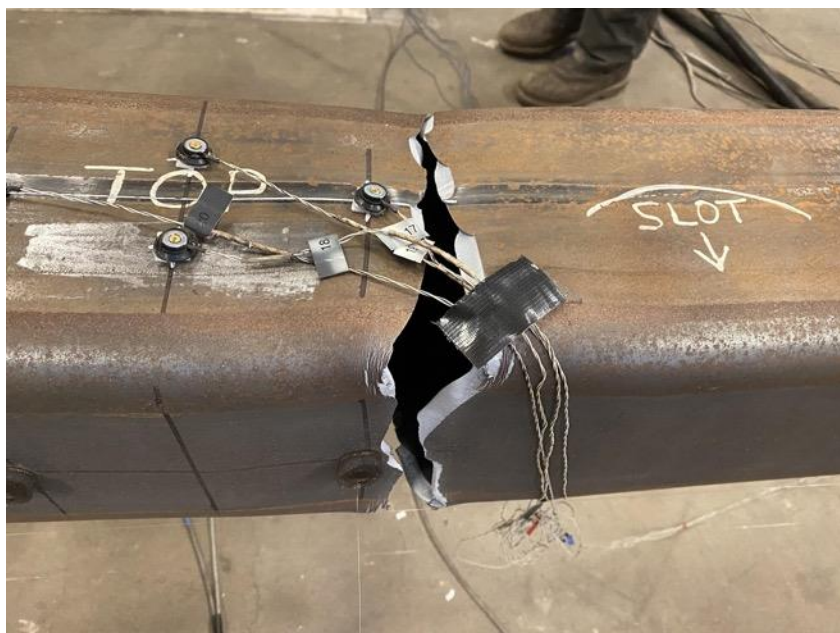
Tearing Through Center of Specimen: 2.75" Cycle 2 T
