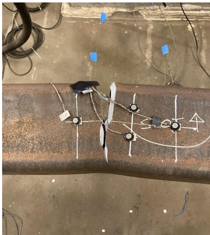
Tearing Through Specimen: 2.75" Cycle 2 T
