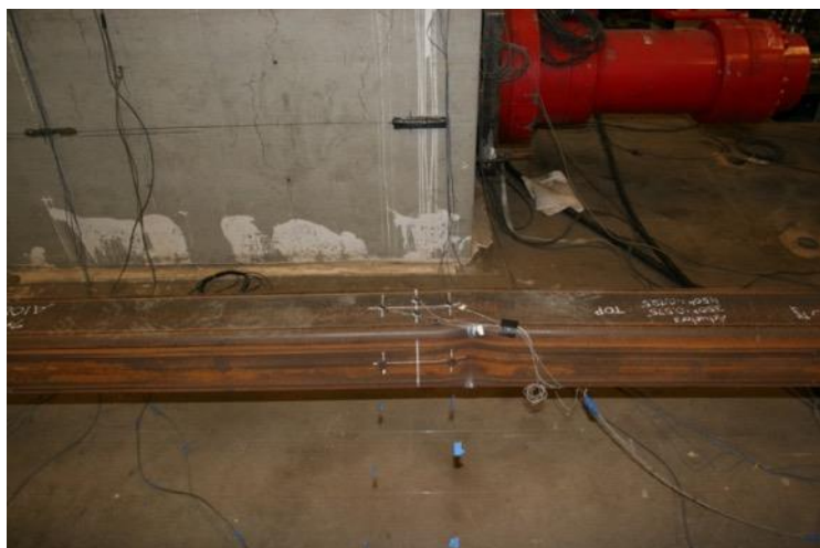
Development of Striations at Center of Specimen: 2.25" Cycle 2 T
