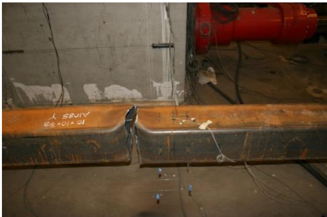
Fractured Specimen: 3.75 Cycle 1 T
