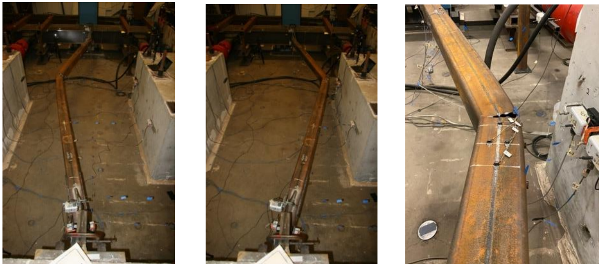
Figure 4.8. Horizontal Buckling Behavior - 6x6x5/16 A500 HSS
