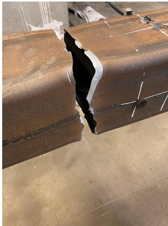
Fractured Specimen: 2.25" Cycle 1 T
