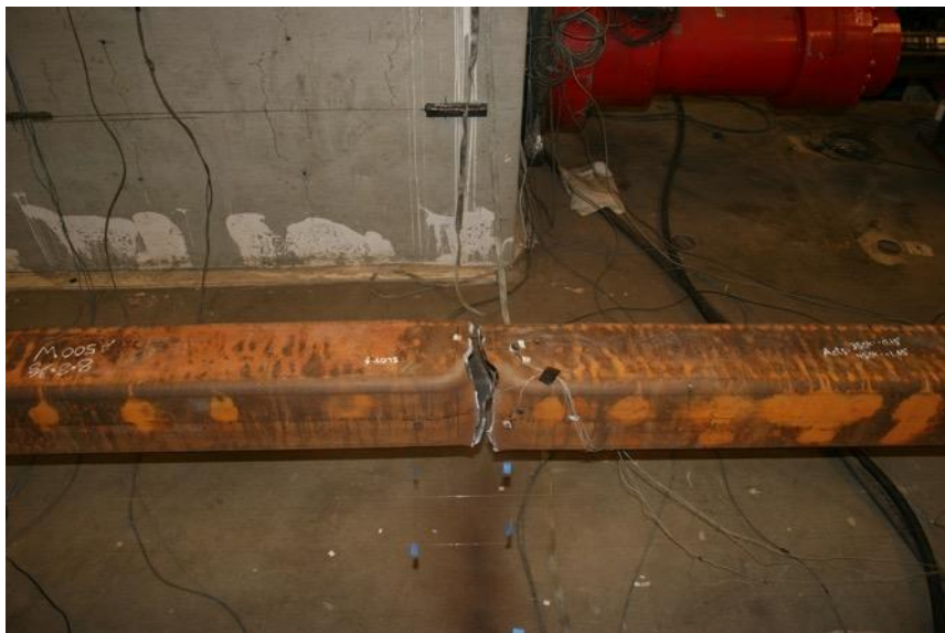
Fractured Specimen: 2.25" Cycle 1 T
