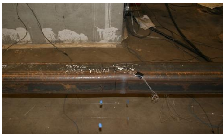
Development of Striations at Center of Specimen: 4.25" Cycle 1 T
