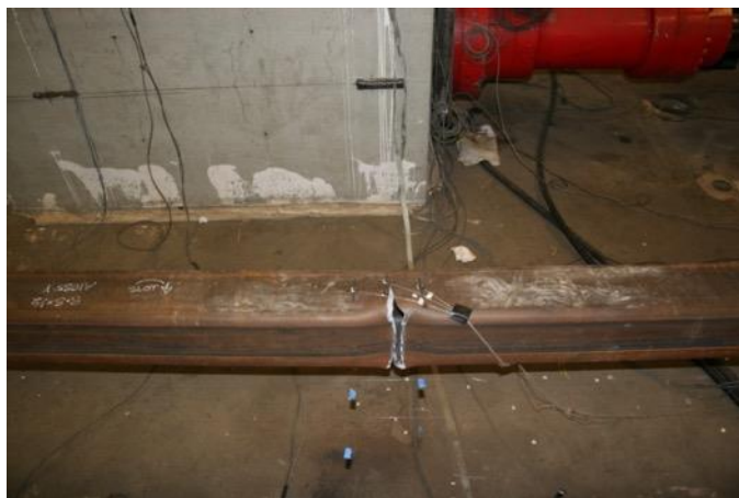
Tearing at Center of Specimen: 3.25'' Cycle 1 T
