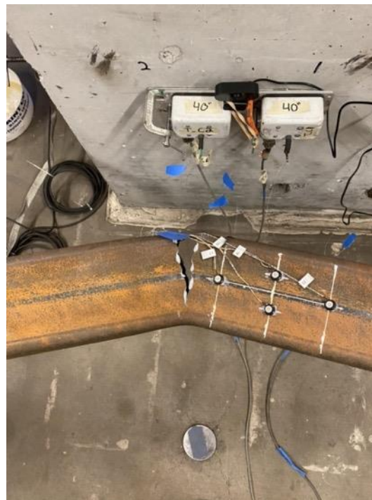
Top View of Tearing in Specimen: Cycle 2 at 3.25" Displacement
