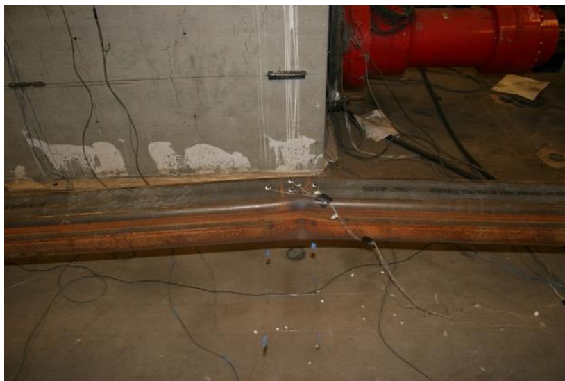
Development of Striations at Center of Brace: 4.25” Cycle 1 T
