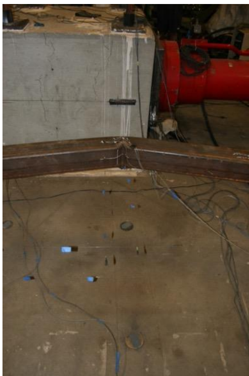
Cupping at Center of Specimen: 3.25" Cycle 2 C
