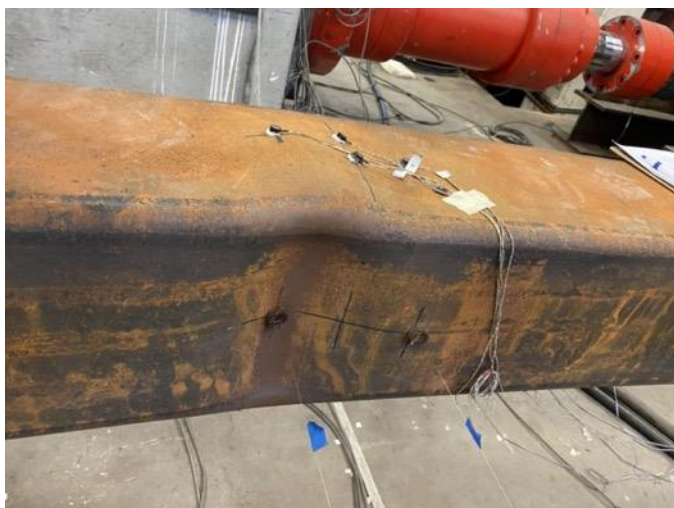
Cupping at Center of Specimen: 1.25" Cycle 1 C
