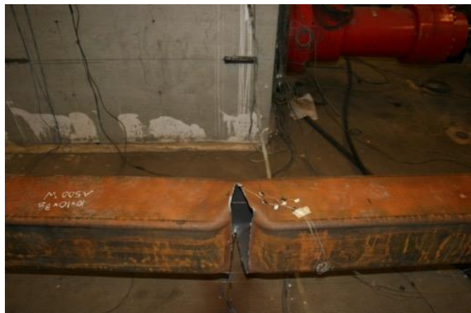
Specimen Immediately Before Fracture: 2.75" Cycle 1 T
