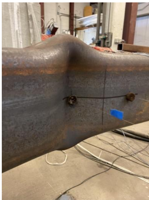
Cupping at Center of Specimen: 2.25" Cycle 1 C
