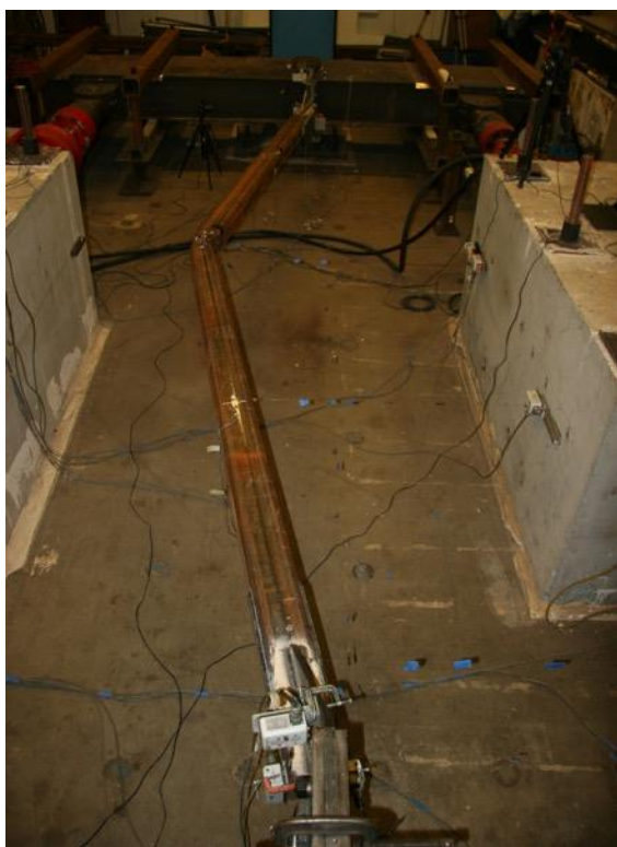
Peak Out of Plane Displacement: 4.25" Cycles
