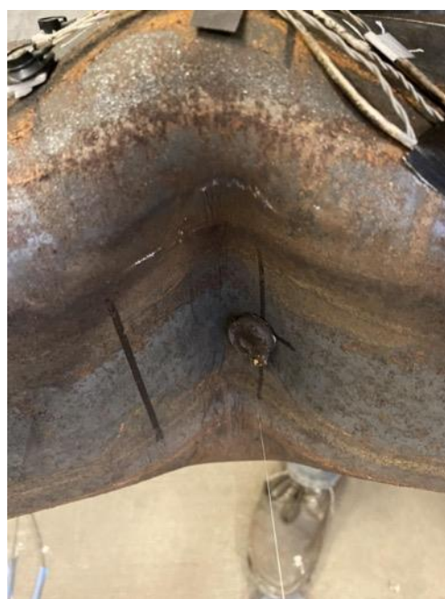
Closeup of Cupping: 4.25" Cycle 1 C
