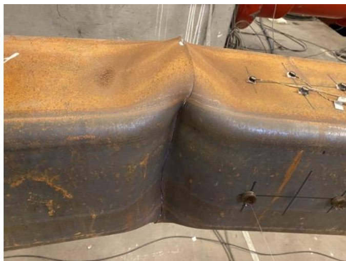
Cupping at Center of Specimen After Tearing: 2.25" Cycle 2 C
