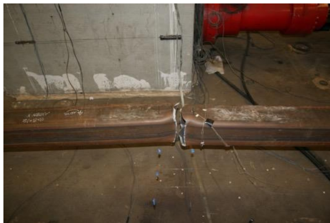
Fractured Specimen: 3.75 Cycle 1 T
