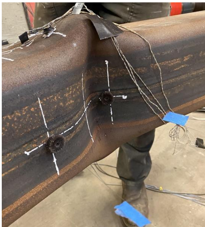
Cupping at Center of Specimen: 2.75" Cycles 1 & 2 C
