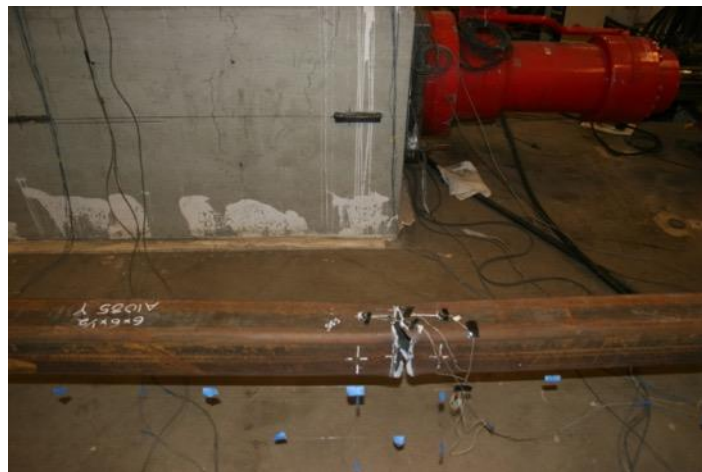
Tearing at Center of Specimen: Second 5.25" Cycle
