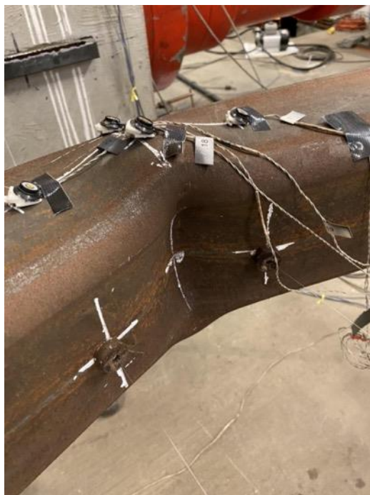
Cupping at Center of Specimen: 4.75" Cycles
