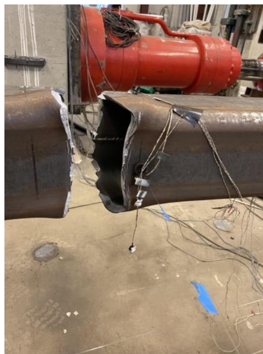
Fractured Specimen after 4.25" Displacement - Cycle 2 T
