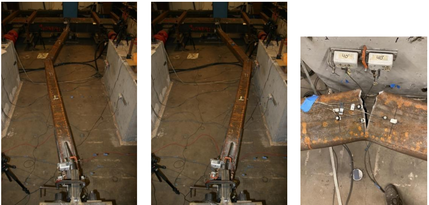
Figure 4.23. Horizontal buckling behavior of the 8x8x1/2 A500 W Specimen
