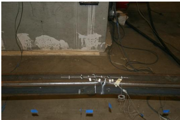
Development of Tearing in Tension - 2nd cycle at 5.75"
