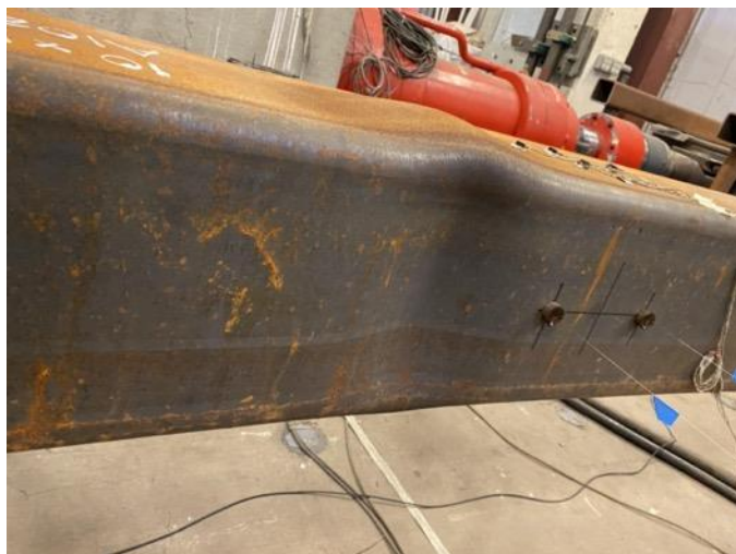
Cupping at Center of Specimen: 1.25" Cycle 1 C
