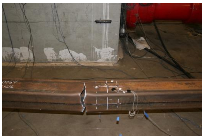
Tearing at Center of Specimen: 2.25" Cycle 1 T
