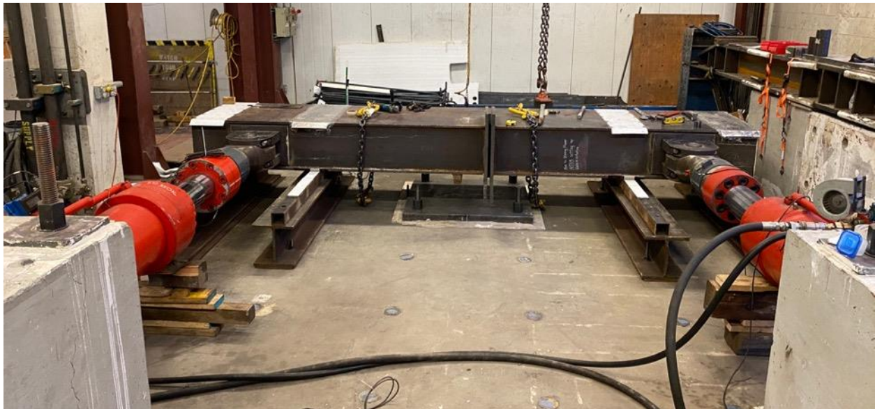
Figure 3.16. Orientation of Actuators and Sliding Beam
