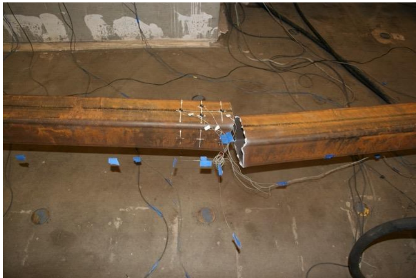
Fractured Specimen: 3.75" Displacement Cycle 1 - Tension
