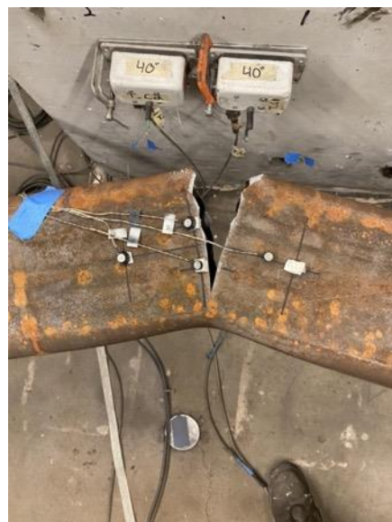
Tearing at Center of Specimen: 3.25" Cycle 1 C
