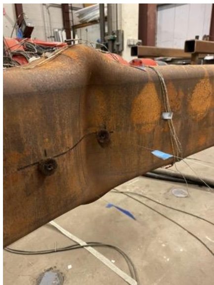
Cupping at Center of Specimen: 1.75" Cycle 1 C
