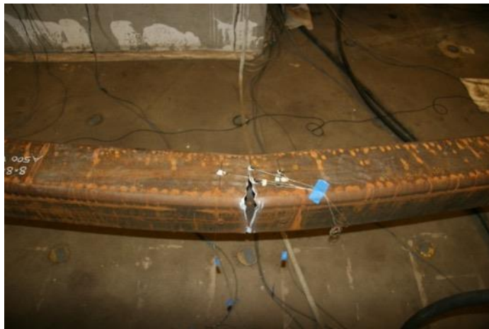
Initiation of Striations and Tearing: 3.25" Cycle 1 T
