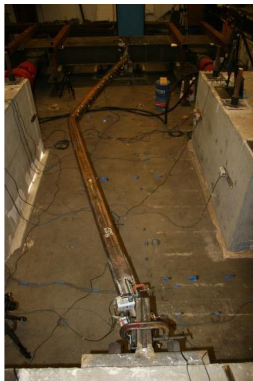
Peak out of plane displacement: 5.25" cycles
