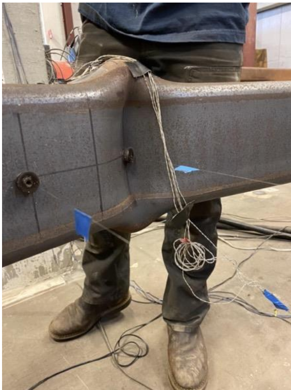
Cupping at Center of Specimen: 2.75" Cycle 1 C
