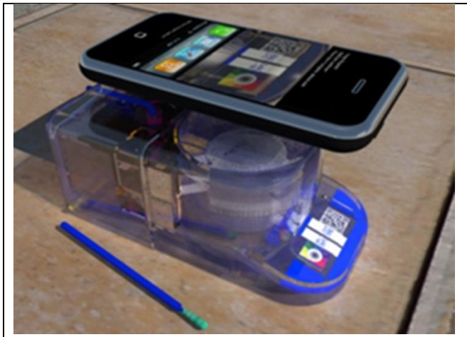
Figure 1: MAD NAAT device. Swab sample obtained from the patient is inserted in the device. The automated assay quantifies nucleic acid sequence of interest. After some time, the cell phone quantifies assay signal. Graphic by Paul Yager.
