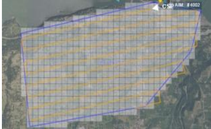
Figure 3.3: Parallel Pattern for search speed of 50kts for a survival raft-sized target (20x20x10ft) resulting in track spacing of 1000ft.
