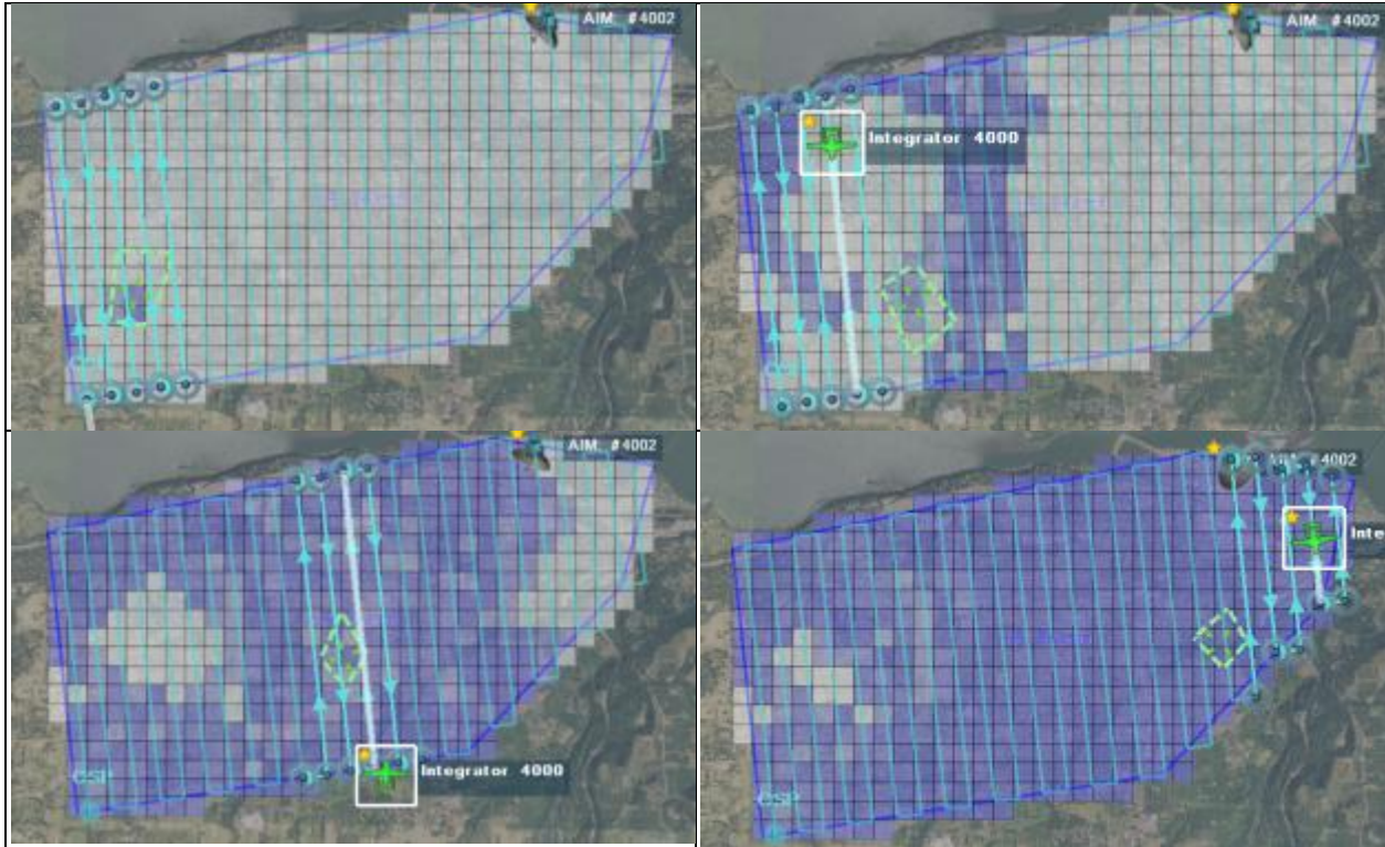
Figure 6.5: Creeping Line search progression snapshots with Occupancy Map-based sensor control algorithm.
