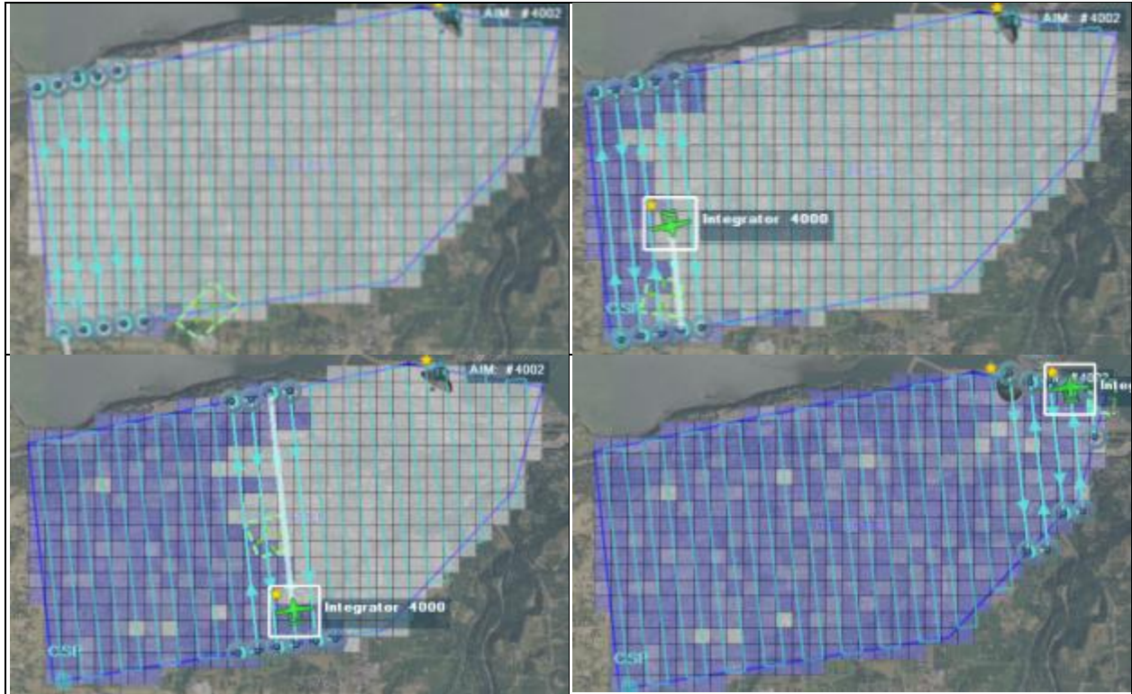
Figure 6.4: Creeping Line search progression snapshots with the pattern-based sensor control algorithm.
