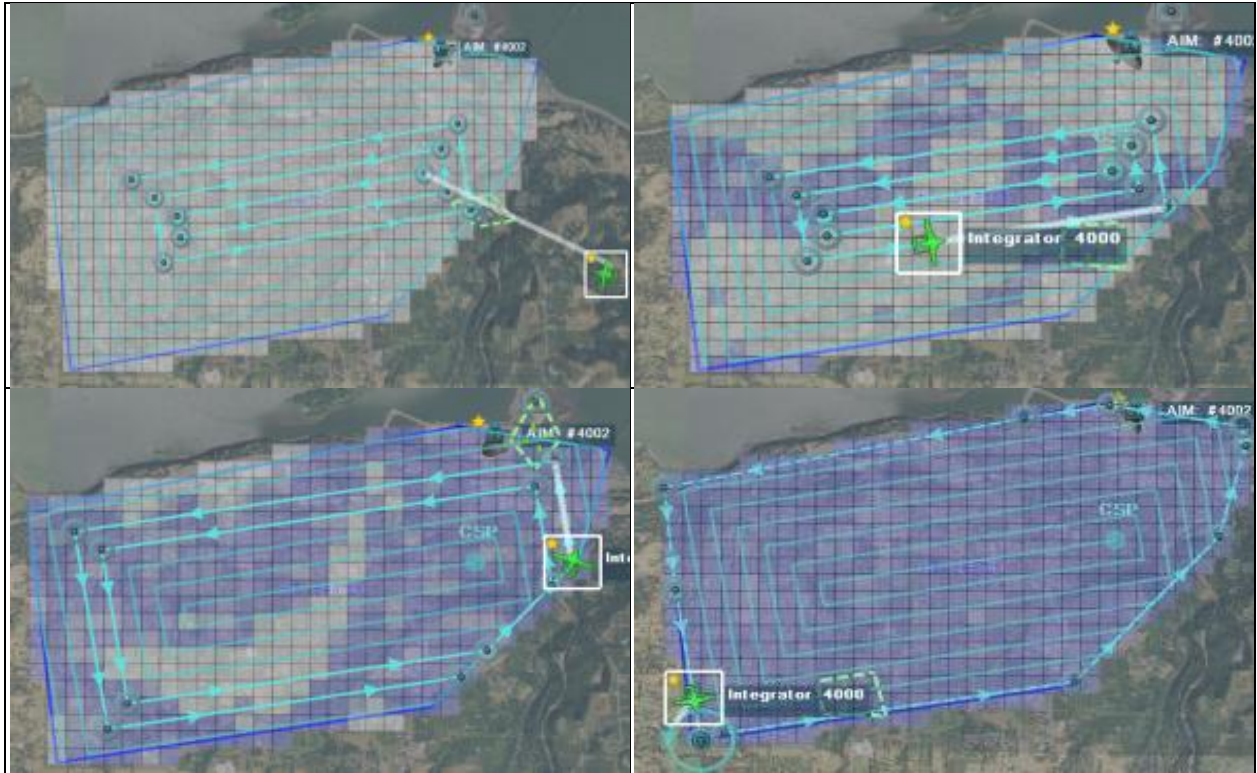
Figure 6.2: Expanding Square search progression snapshots with the Occupancy Map-based sensor control algorithm.
