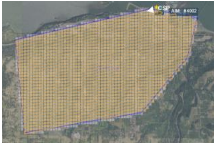
Figure 3.2: Parallel Pattern for search speed of 50kts for a car-sized target (16x6x6ft) resulting in track spacing of 270ft.
