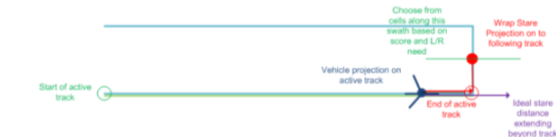
Figure 4.3: Pattern-based sensor control while approaching cross leg.
