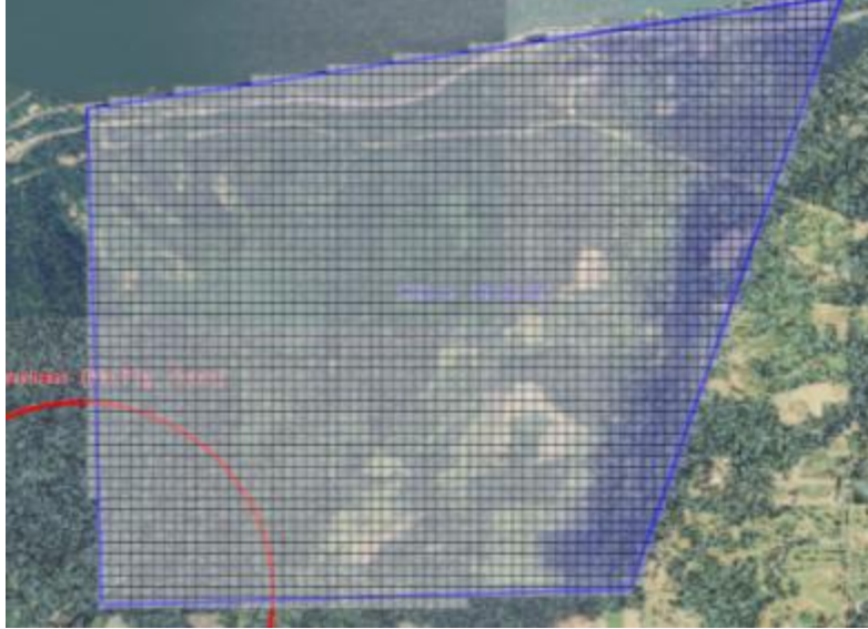
Figure 3.1: Occupancy Map visualization. Purple cells have lower target probabilities.
