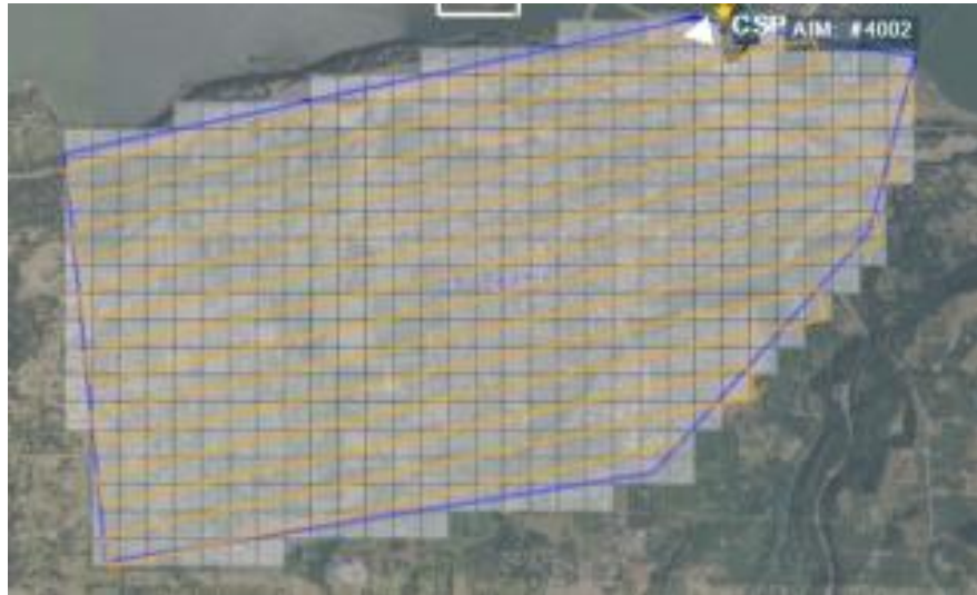
Figure 3.4: Parallel Pattern for search speed of 90kts for a survival raft-sized target (20x20x10ft) resulting in track spacing of 600ft.
