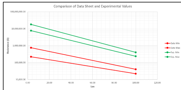
Figure 14: LDR performance experimental and datasheet comparison
