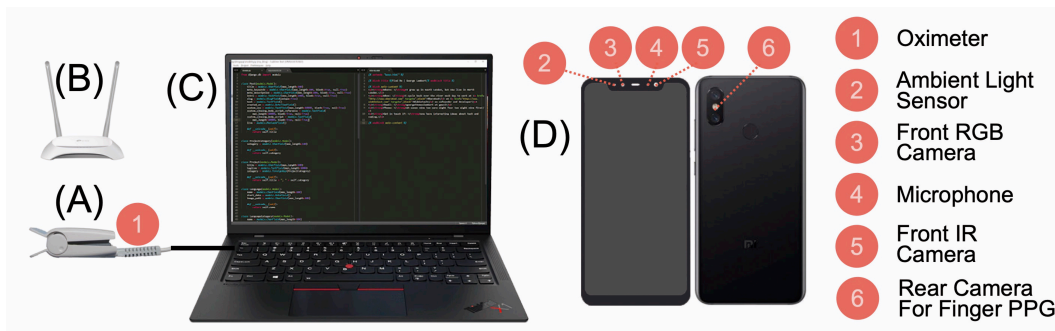
Figure 4.6: The hardware setup includes (A) an oximeter for gold standard contact PPG measurement, (B) a WiFi router for wirelessly streaming the smartphone’s data to the desktop, (C) a desktop with the back-end server for collecting and synchronizing data, and (D) a Xiaomi 8 / iPhone 11 smartphone providing signals from multiple built-in sensors for physiological sensing.
