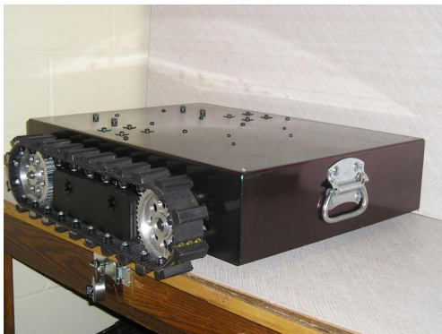
(c) Tank inspection robot by Kalra et al al)
