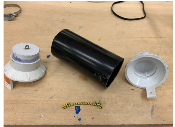
Figure 1: Basic pieces of the prototype Niskin bottle, featuring an open tube, two end caps and an elastic connection chord.
