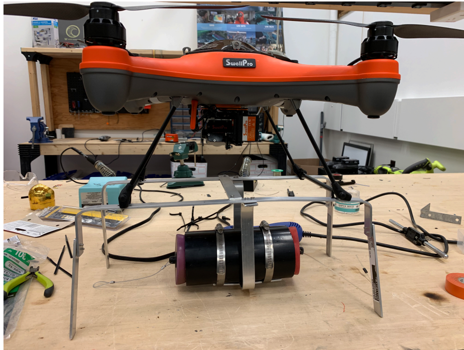
Figure 3: First prototype of landing gear with Niskin bottle mounted.
