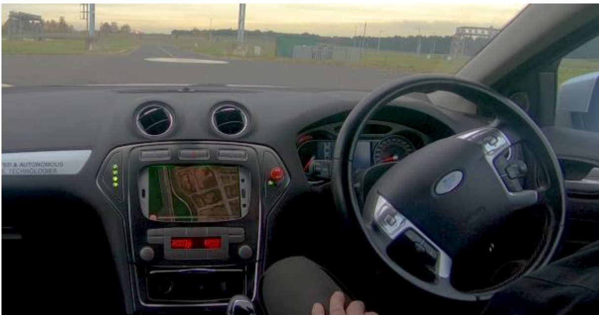
Figure 11. NGV during test with display showing NGV position, path and real/virtual test participants
