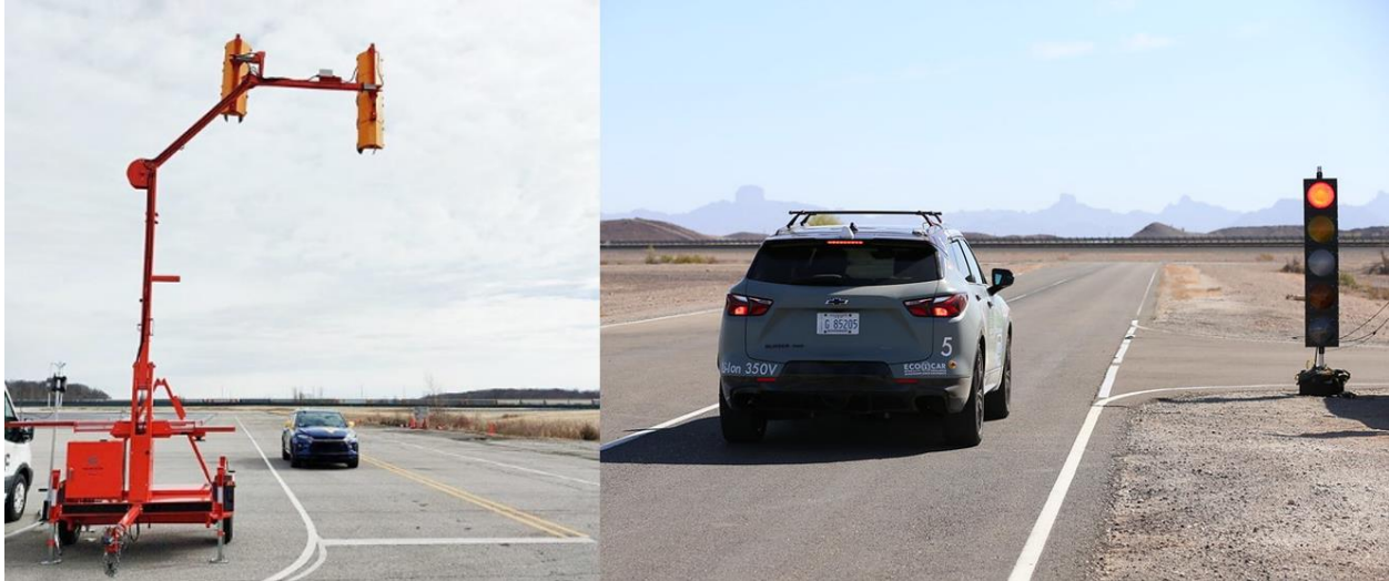
Figure 49. Construction zone signal system at TRC (left) and smaller single signal at GM (right)
