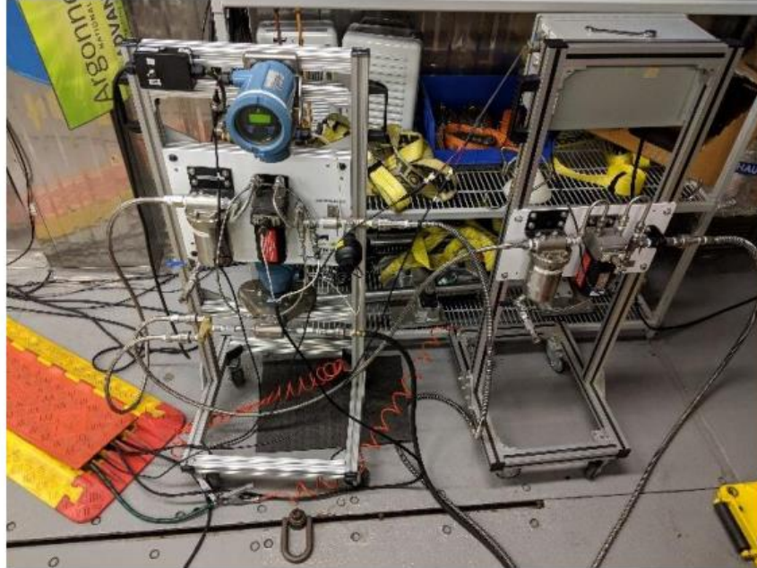
Figure 41. Direct Fuel Flow Measurement Coriolis and Fuel Scale Instruments
