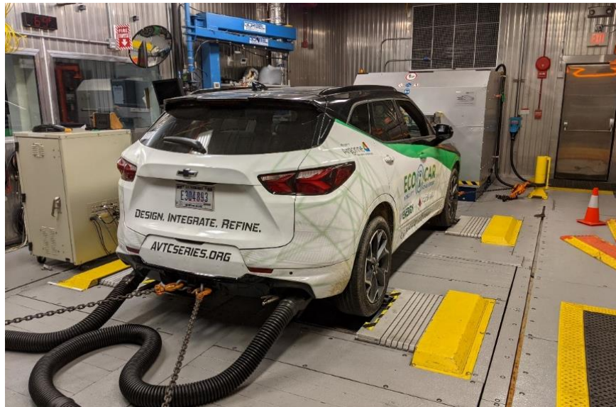
Figure 38. Argonne Blazer Setup on 4WD Chassis Dynamometer for University ACC Cycle Testing
