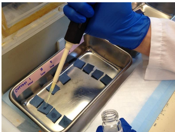
Figure A-7. Loading radiolabeled compound to fabric sample.
