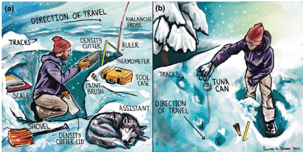
Figure 2.2. Illustration of field sampling protocol. We excavated a snow pit parallel to the animal's direction of travel and conducted observations, including measuring density of the top 30 cm (a; AvgDens ), determining hand-hardness across the full pit's depth ( AvgHH ), quantifying thickness and depth of ice layers ( IceTop and TotalIce ), and measuring surface penetrability via tuna can drops (b; AvgTuna ). The string under the tuna can measured 50 cm, the height at which the can was dropped from. Illustration by Sarah K. Glaser.
