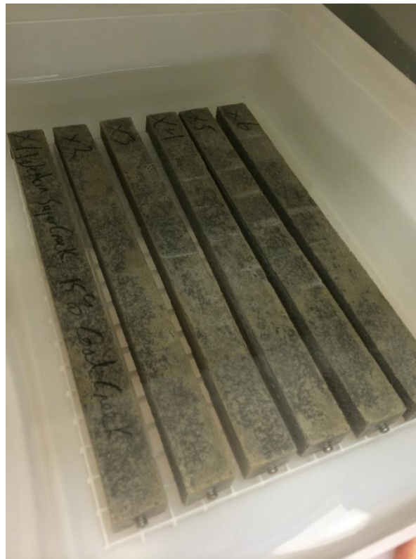
Blended Cement being tested for sulfate resistance Source: Author
