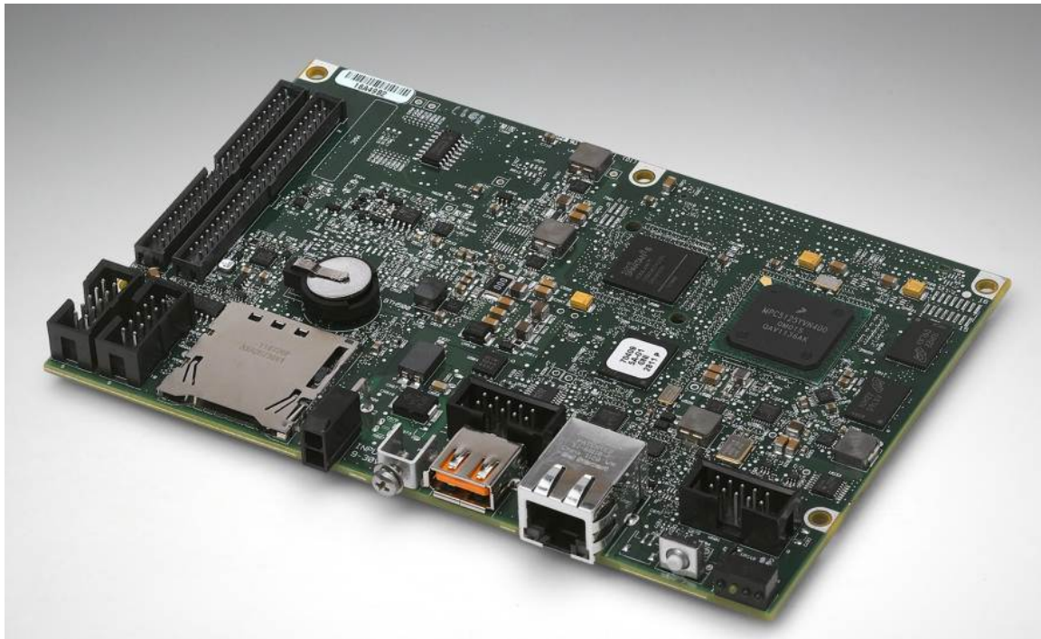
Figure 3.2: The National Instruments 9632 sbRio, picture from NI.com
