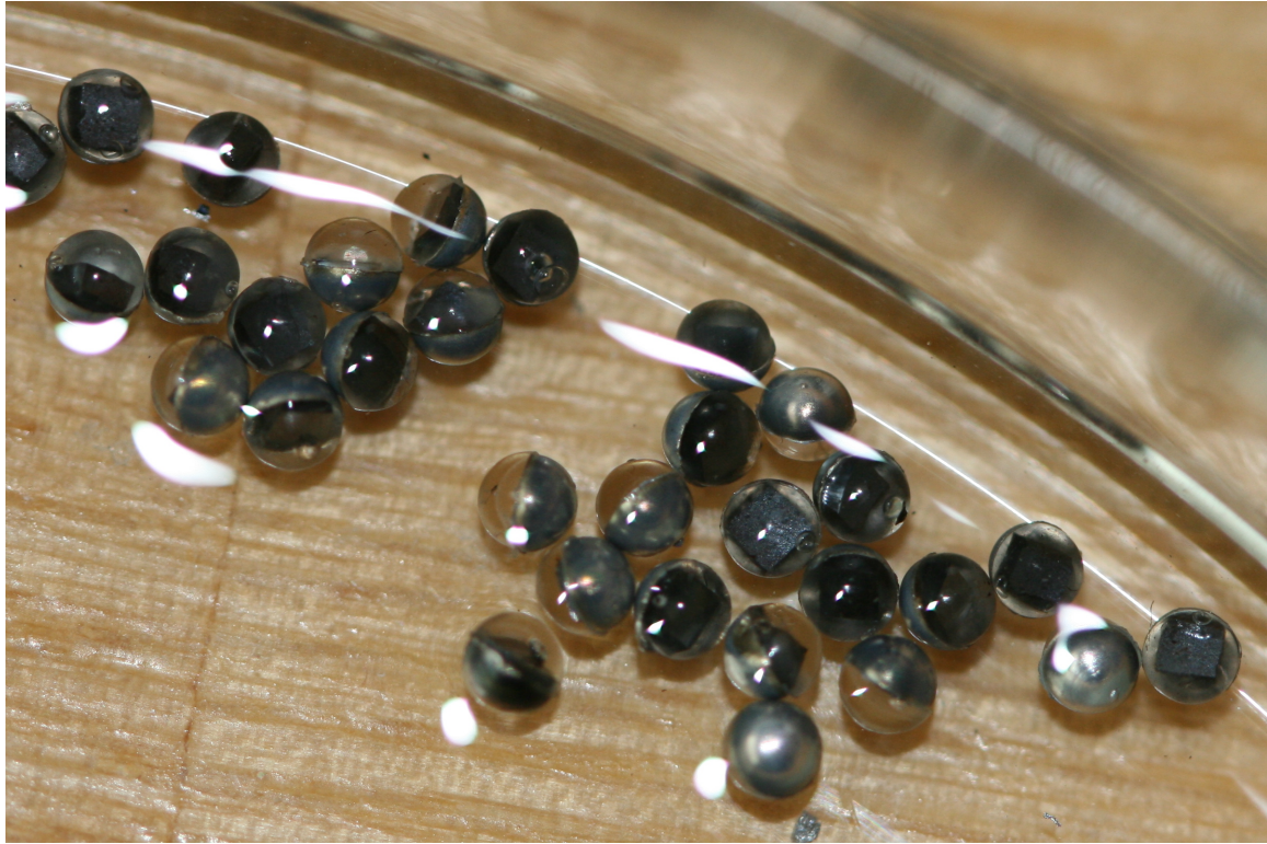
Figure 3.49 Epoxy drops of 1.75mm diameter, with mirror layers on them, released from the mold
