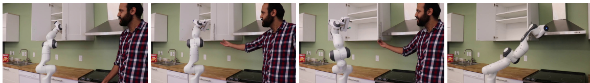
Figure 5.6: Reactivity. The door handle location is displaced during execution and the robot can be seen to adapting to the new target.
