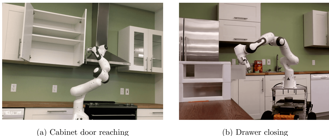
Figure 4.1: Target reaching, which requires the a certain point of a robot to reach a target in a particular way, is an important component of a lot robotics problems. (a) The robot reaches the cabinet door handle with its gripper from inside the cabinet. (b) The robot uses end-effector to close a drawer.
