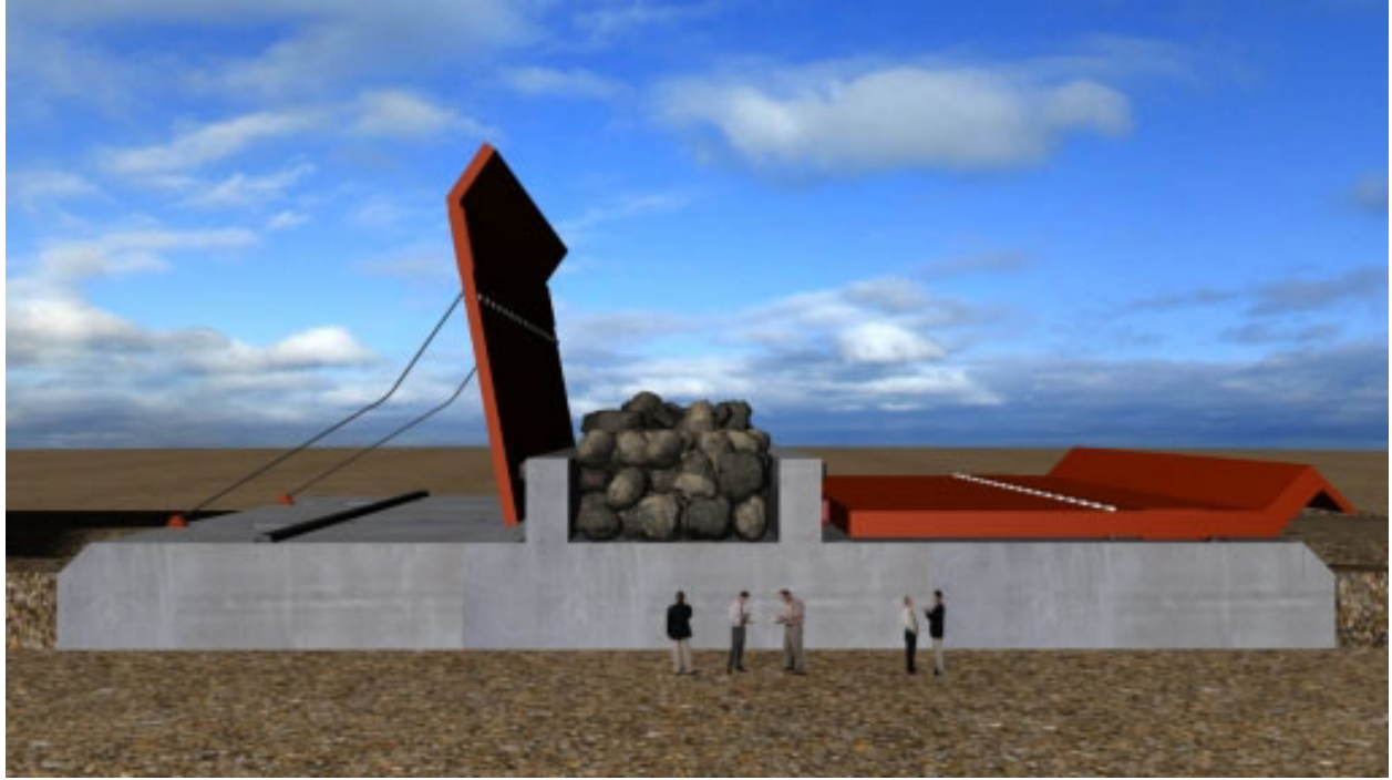
Figure 022: Twin Wing Tsunami Barrier Concept
