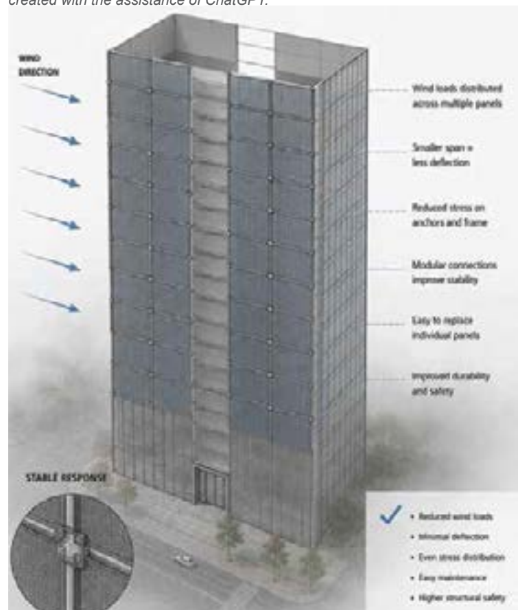
Fig 3.10: Proposed modular system. Source: Illustration by the author, created with the assistance of ChatGPT.
