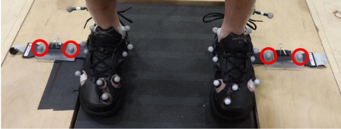
Figure 15 – Image of static markers used to locate the position of the insoles relative to the location of the feet markers. Markers defining position of insole circled in red.
