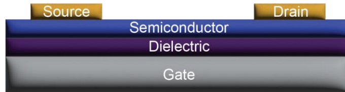
Fig. A1 | Diagram of bottom gate top contact architecture organic field-effect transistor (OFET). Gate is typically silicon, dielectric is a siloxane monolayer, semiconductor is the active layer, and source and drain are gold electrodes.
