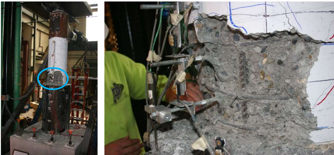
Figure 4.111. Specimen 30-21-LD Increased Spalled Region at 5.5% Drift
