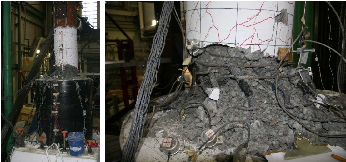
Figure 4.57. Final State of Specimen 48-21 after 9.7% drift
