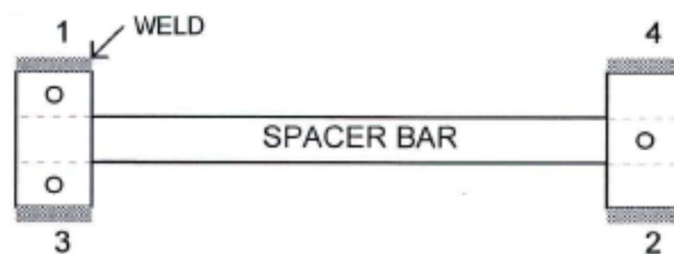
Figure 3.14. Welding Sequence for the Mounting Blocks (Geokon, 2010)
