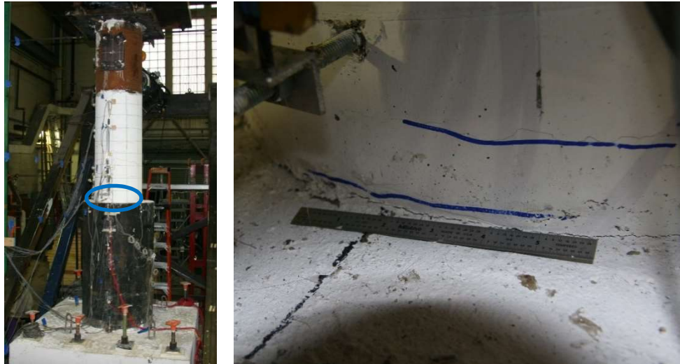
Figure 4.13. Specimen 30-21 Interface Cracks on Southern Face at 0.9% Drift
