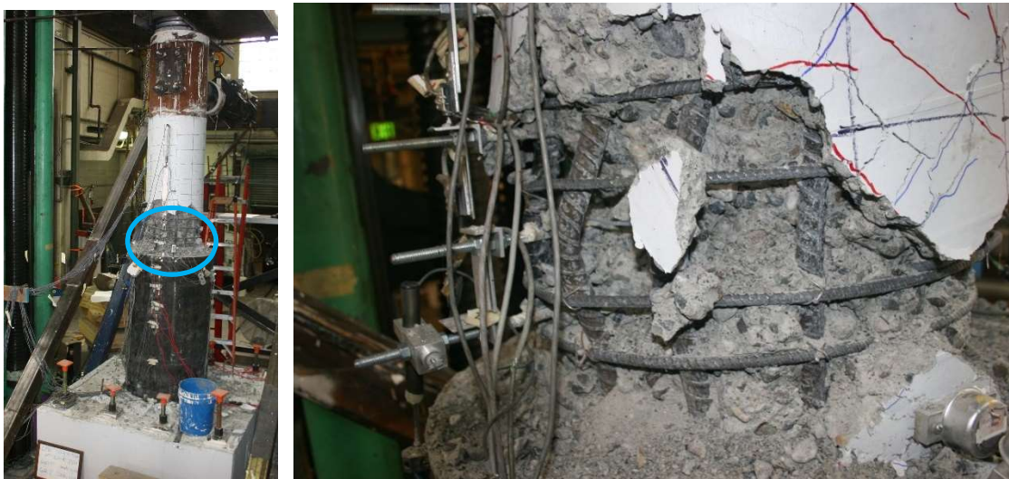
Figure 4.89. Specimen 30-21-R Base of Column at 9.3% Drift
