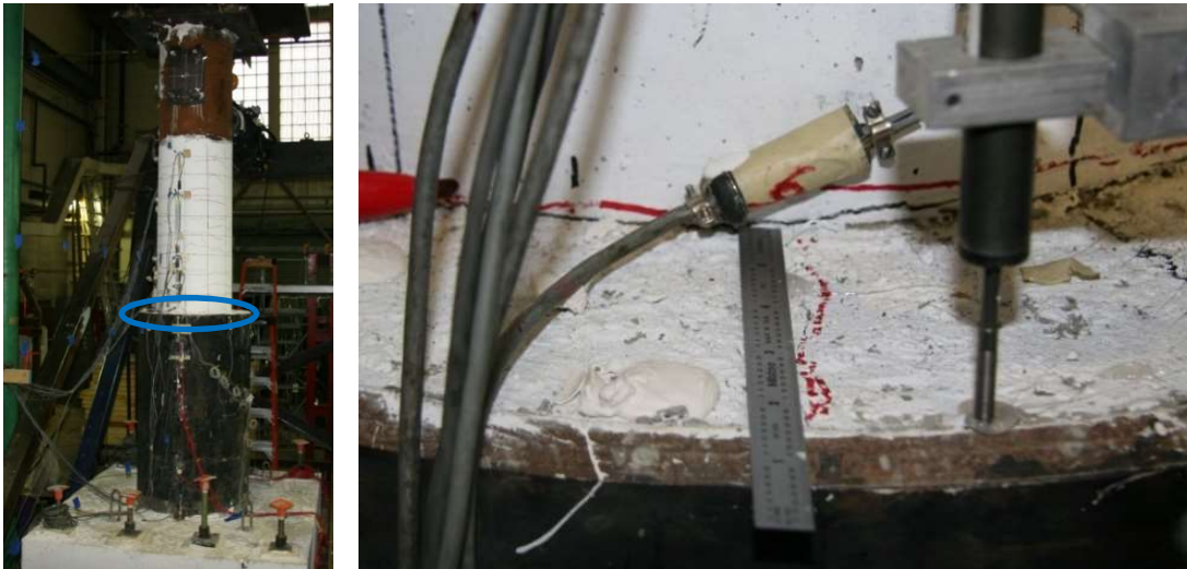
Figure 4.15. Specimen 30-21 Radial Cracks on North Face of Column
