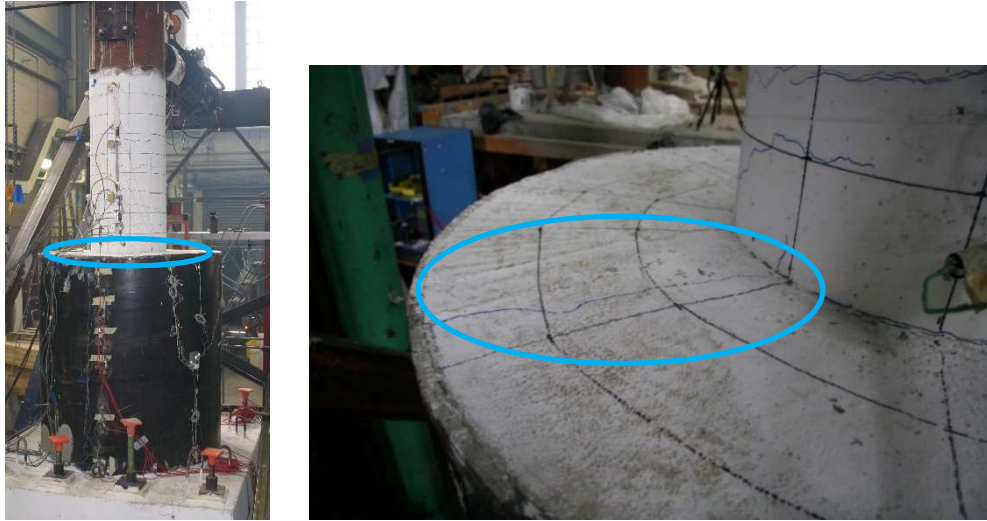
Figure 4.39. Specimen 48-21 Radial Cracks on Top of Pile Concrete at 0.8% Drift
