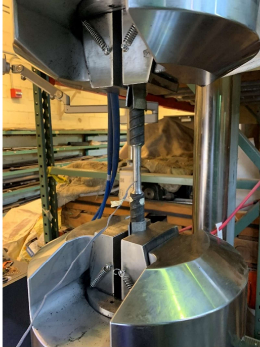
Figure 3.6. Reinforcement Tensile Test Setup
