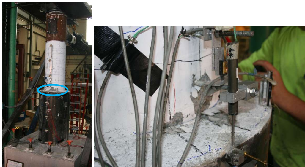
Figure 4.101. Specimen 30-21-LD 1 st Spalled Region on Northern Column Face at 2.4% Drift
