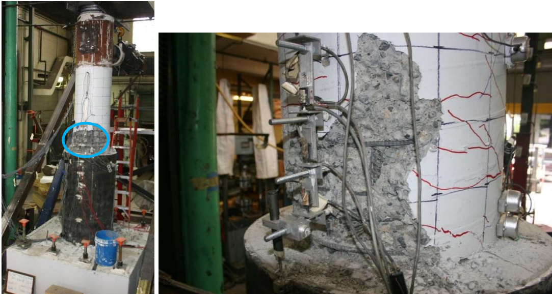
Figure 4.85. Specimen 30-21-R South Face Buckled Longitudinal Reinforcement Bars at 8.9% Drift
