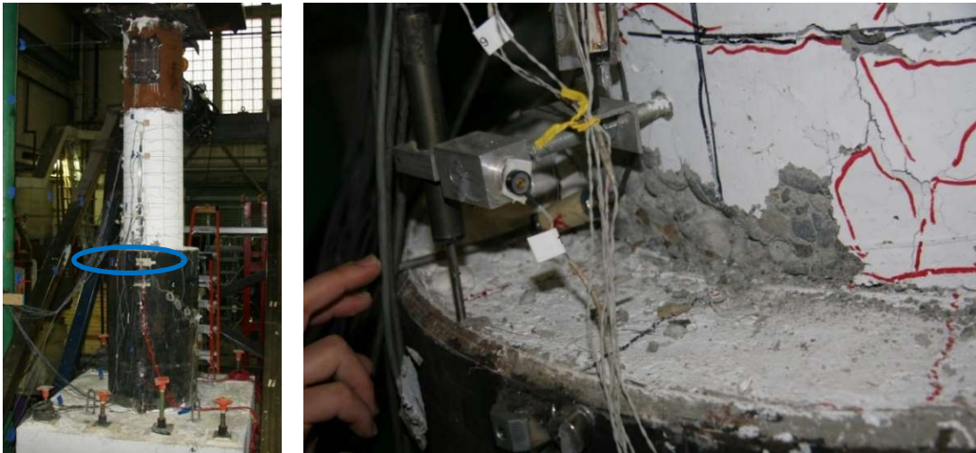
Figure 4.18. Specimen 30-21 Initial Spalled Region on North Face at 2.2% Drift
