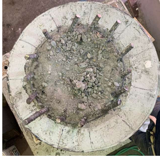
Figure 4.91. Top of Specimen 30-21-R Pile with Column Removed
