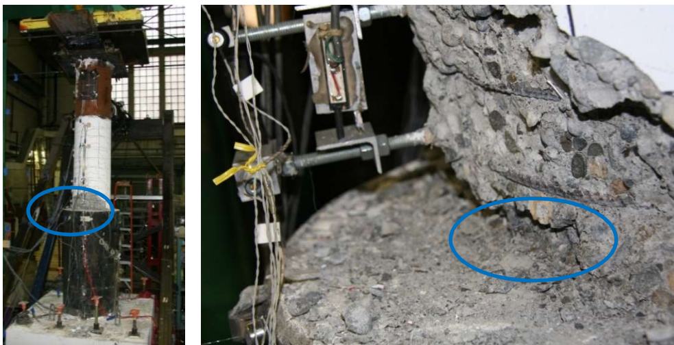
Figure 4.24. Specimen 30-21 Exposed Longitudinal Reinforcement on South Face
