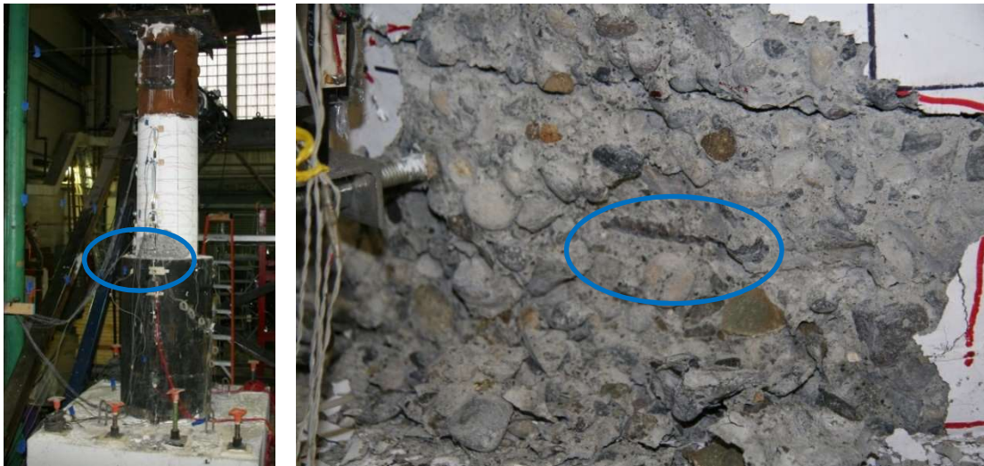
Figure 4.21. Specimen 30-21 Spalled Region on Northern Column Face at 3.7% Drift
