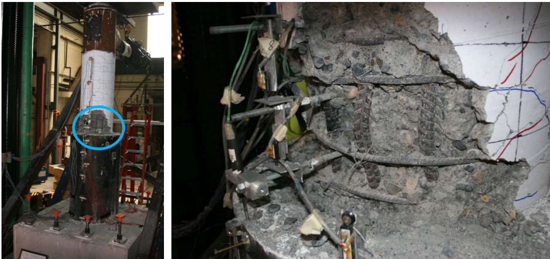
Figure 4.117. Specimen 30-21-LD Northern Face of Column after 10 cycles at 5.5% drift
