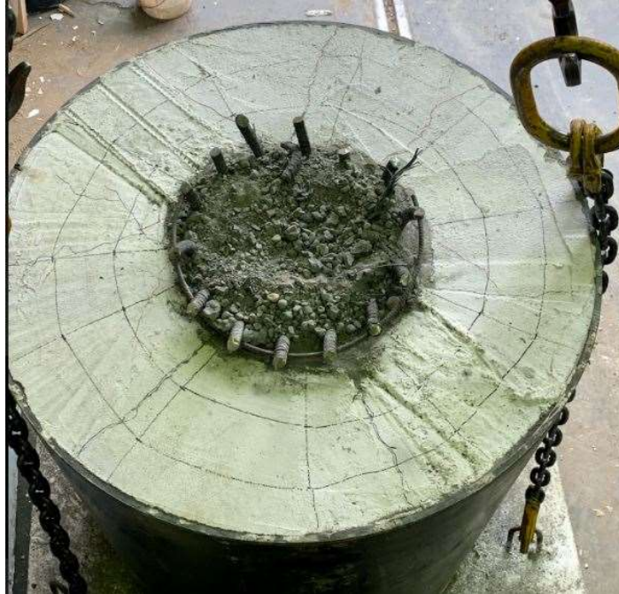
Figure 4.58. Top of Specimen 48-21 Pile with Column Removed
