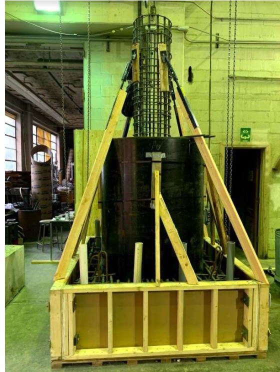
Figure 3.4. Specimen Reinforcement a) Specimen Elevation and Reinforcement and b) Specimen 48-21 Completed Reinforcement Cage
