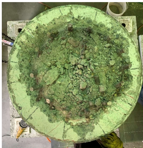
Figure 4.121. Top of Specimen 30-21-LD Pile with Column Removed
