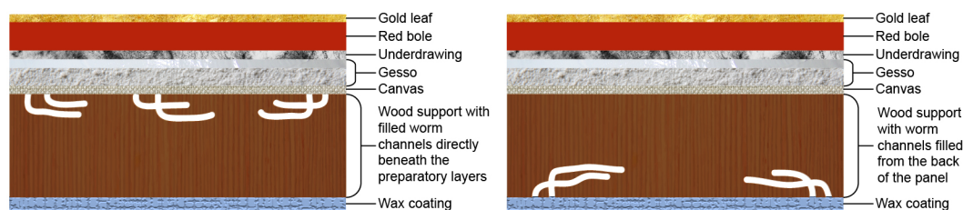
Figure 6.8. Diagrams of possible woodworm channel spatial arrangement within the Madonna and Child's wood support. Left: the channels would have to have been filled prior to the application of the canvas and gesso (the preparatory layers), indicating the damage occurred before the painting’s creation. Right: the larvae entered from the back of the panel, likely after the artwork’s creation.
