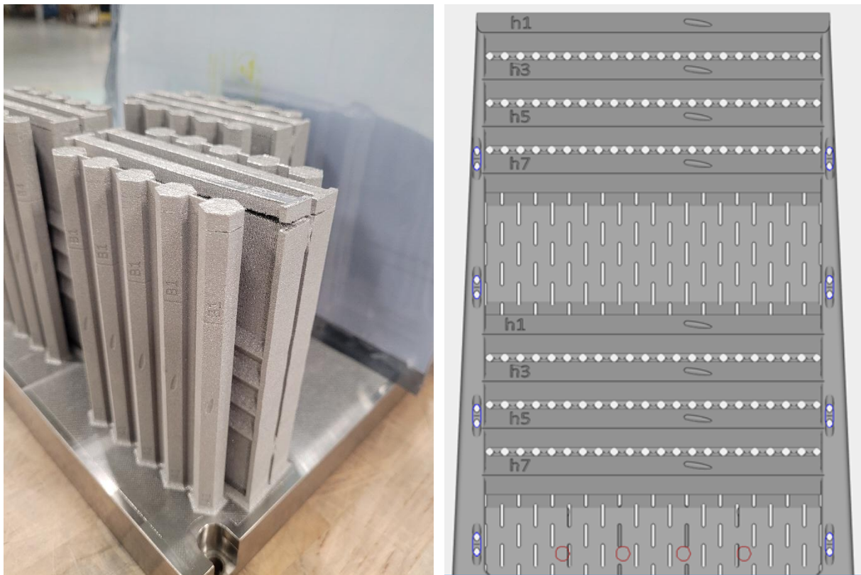
Figure 2.17: Demonstration of the importance of support structures. The left image shows a delamination of layers due to the compressive stress created by the solidification and cooling of the horizontal coupon melt pool. The right image shows a model of the horizontal coupon assembly, with a tapered support frame to provide rigidity and resist the compressive stresses, and intentionally designed support between horizontal coupons to provide support without increasing the compressive stresses.
