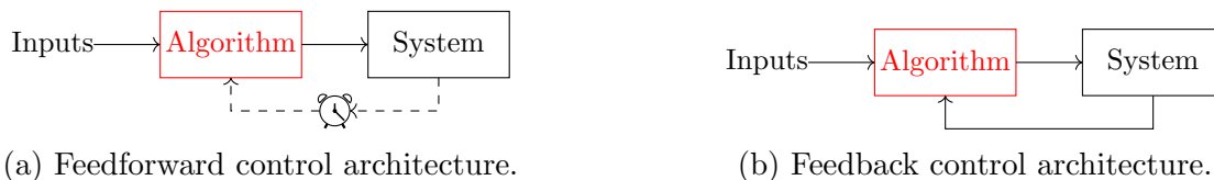
Figure 1.2: Comparison of feedforward and feedback algorithms in relation to the system being controlled.
