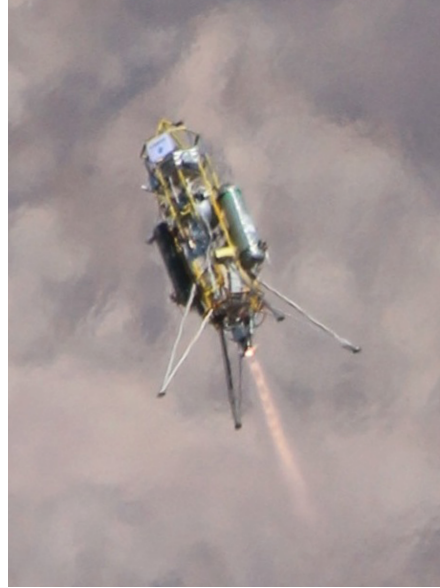
Figure 6.12: A Xombie technology demonstrator from Masten Space Systems, Mojave, Calif., ascends from its pad at Mojave Air and Space Port on a test for NASA's Jet Propulsion Laboratory. The vehicle is a vertical-takeoff, vertical-landing experimental rocket. It is being used in collaboration with NASA Dryden Flight Research Center to evaluate performance of JPL's Fuel Optimal Large Divert Guidance (G-FOLD), a new algorithm for planetary pinpoint landing of spacecraft. Image and caption credit: NASA/Masten [172].
