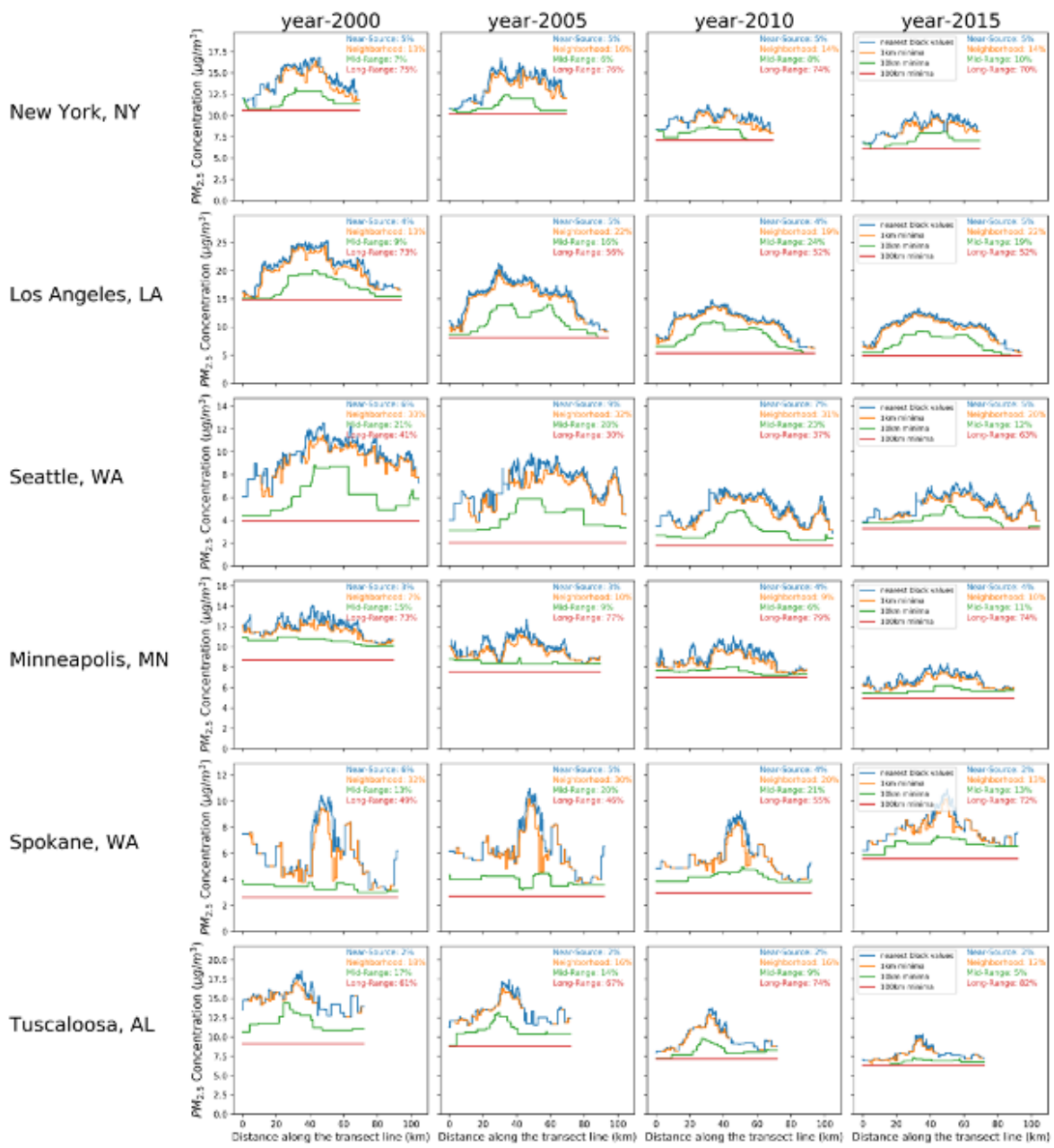
Figure 2.14: Multiple years (2000, 2005, 2010, 2015) PM 2.5 transect line decomposition plots and average contributions of four components (upper right of each subplot) for six cities.
