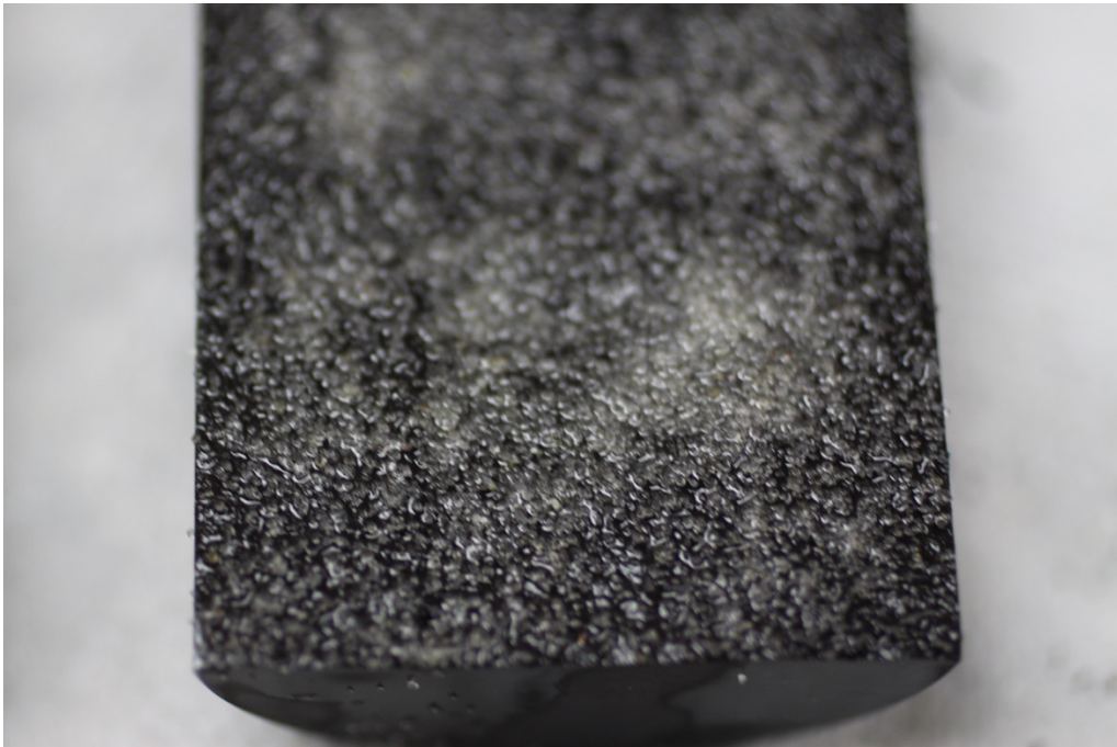
Figure 8: Image of one of the cores with proppant applied to the fresh fracture. Image by Johnathan Moore, 2017.
