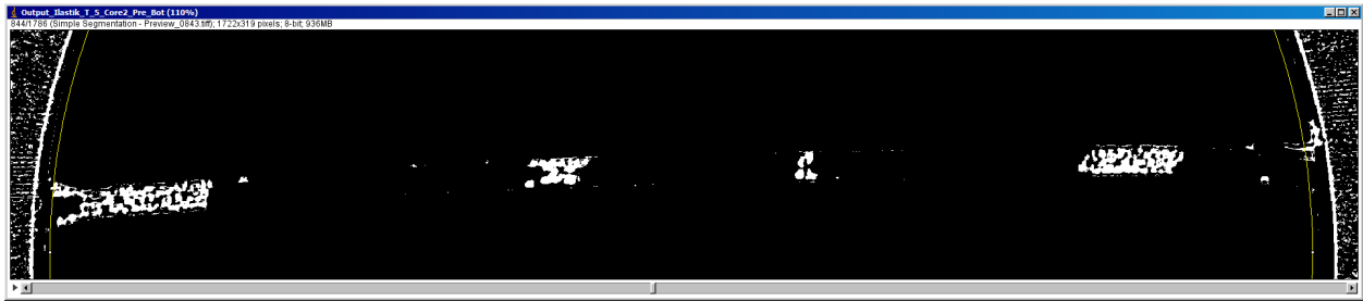
Figure A6: The segmented image from Ilastik in ImageJ. Following the work flow I created (Table 1), an ROI (region of interest; thin yellow line) was created to crop out the are outside of the rock core. In the center, in white, are the proppant grains in the fracture.
