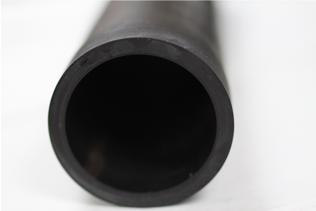
Figure 7: Image of one of the Buna-N rubber tubes used in both tests. Rubber tubes were used due to their lower attenuation for CT scanning than metal casings. Image by Johnathan Moore, 2017.
