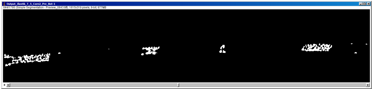
Figure A8: Continuing to follow the workflow from Table 1, the image shows the proppant after removing the outliers.
